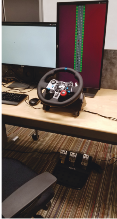
Figure 4.4: The system used for collecting driving performance data from human testers: A logitech driving wheel, acceleration and braking paddles, and a chair.
