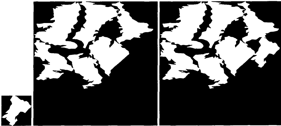
Figure 4.15: The binary mask of the piece (left) is to be inserted into the global occupancy mask (middle). The texture coordinate offset for the piece is obtained by finding the first available position for the piece, illustrated in the updated occupancy mask (right).
