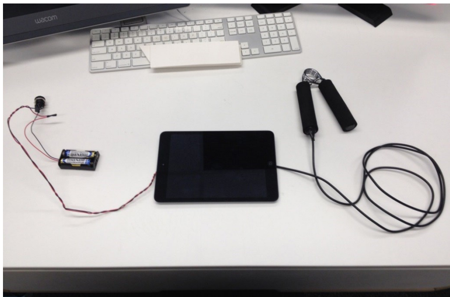
Figure 1: Device with hand grip, iPad and vibrating disk motor attached to the back
