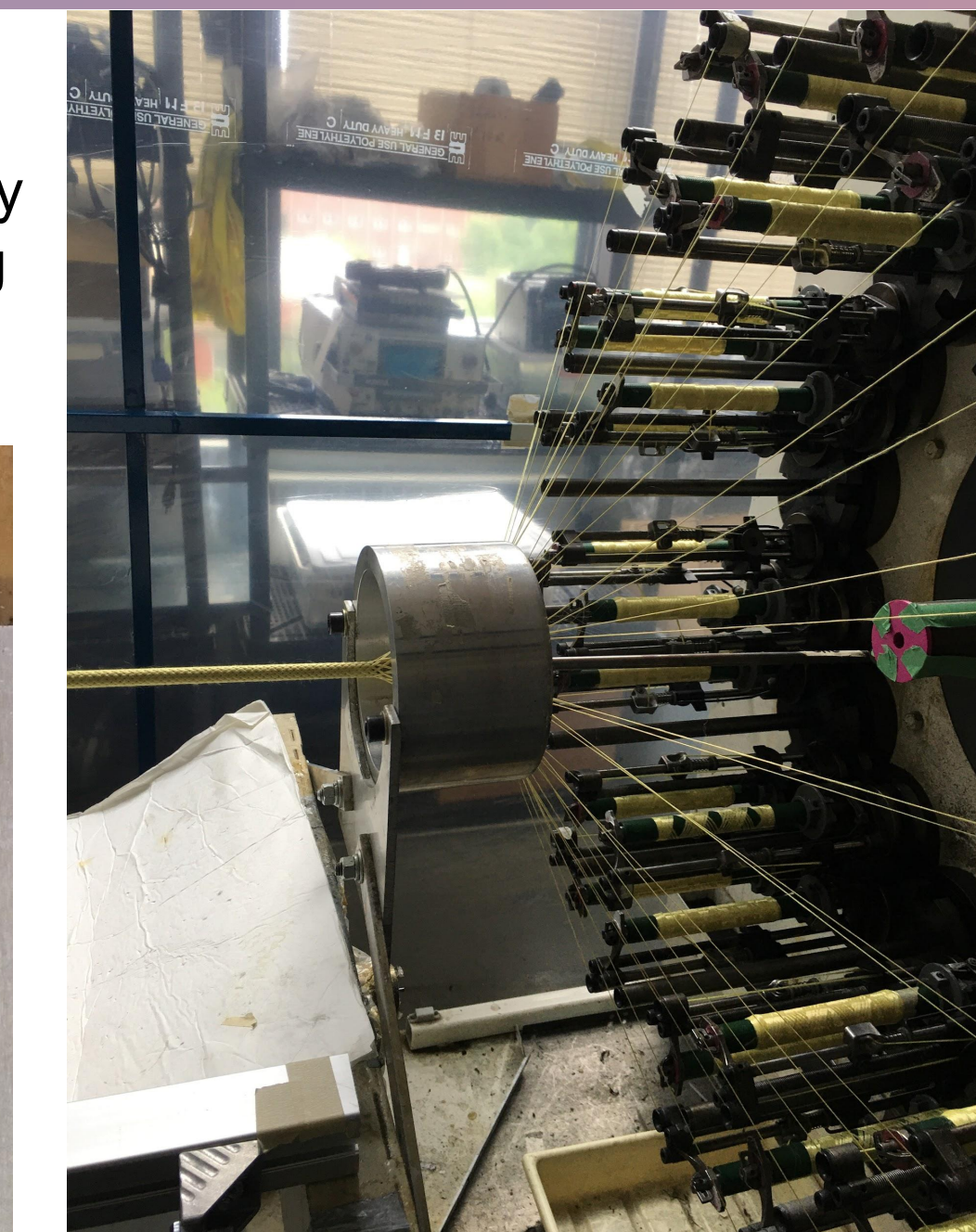
Figure 9: Process of covering assembled racket with braided preforms
