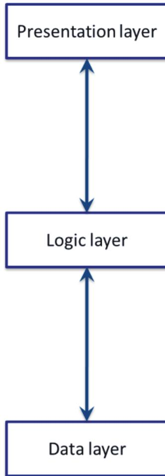
**Figure 1.6.** CDSS as a three-tier architecture. This multi-layered approach to software development consists of interconnected presentation, logic and data storage layers to optimize speed, consistency and applicability of data transfers.
