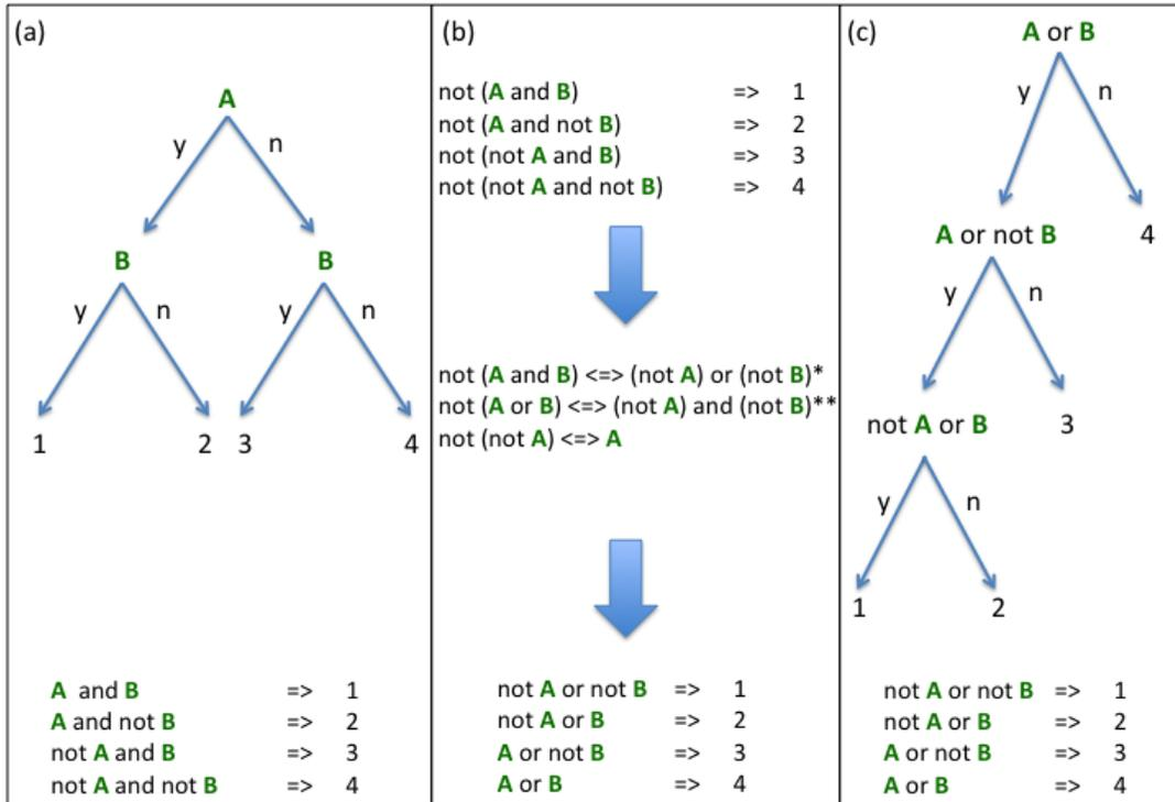
**Figure 3.3.** Trade-off of simplicity and depth when converting a PGENI tree to augmented FFT format. (a) The PGENI tree, with cue-conditions leading to each outcome; (b) Transformation of cue-condition formulae to allow each outcome to be accessible via ‘no’, as required in augmented FFT format. This is done by applying De Morgan’s (\*De Morgan #1; \*\*De Morgan #2) and standard logic laws; (c) Corresponding augmented FFT.
