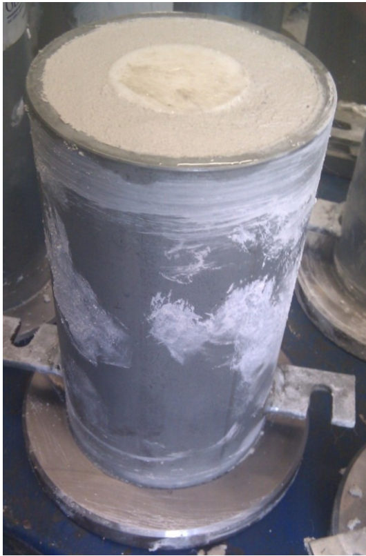
Figure 3.4 Preparation of hollow cylindrical specimen
