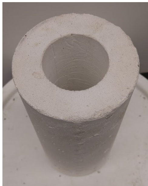
Figure 3.5 Extracted hollow cylinder for permeability tests
