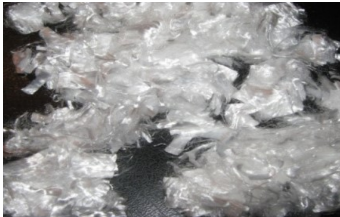
Figure 3.2 Polypropylene micro-fibres used in this study
