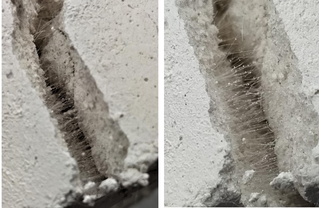
Figure 4.6 Fibres in mortar
