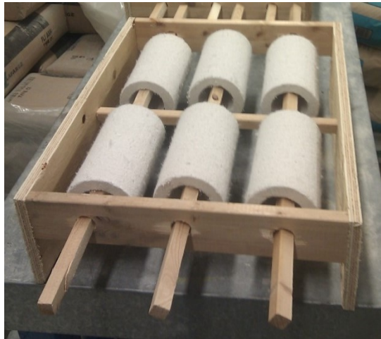
Figure 6.14 Hollow Cylinders Supported in a Wooden Cage
