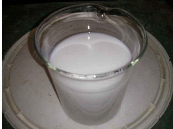
Figure 6.12 Nano-lime suspension, placed in a glass jar, that was used in this study
