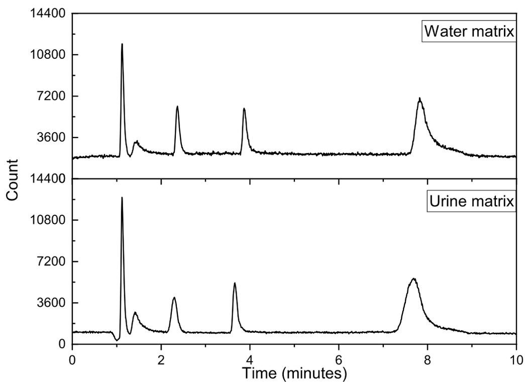
**Figure 2.12** 1  $\mu\text{g/L}$  concentration of arsenic standards in water matrix and urine matrix. The two matrices were compared to determine if the more acidic pH of urine, and addition of other contaminants found in urine (e.x. chloride, salt, uric acid, urea) could affect the detection of arsenic.
