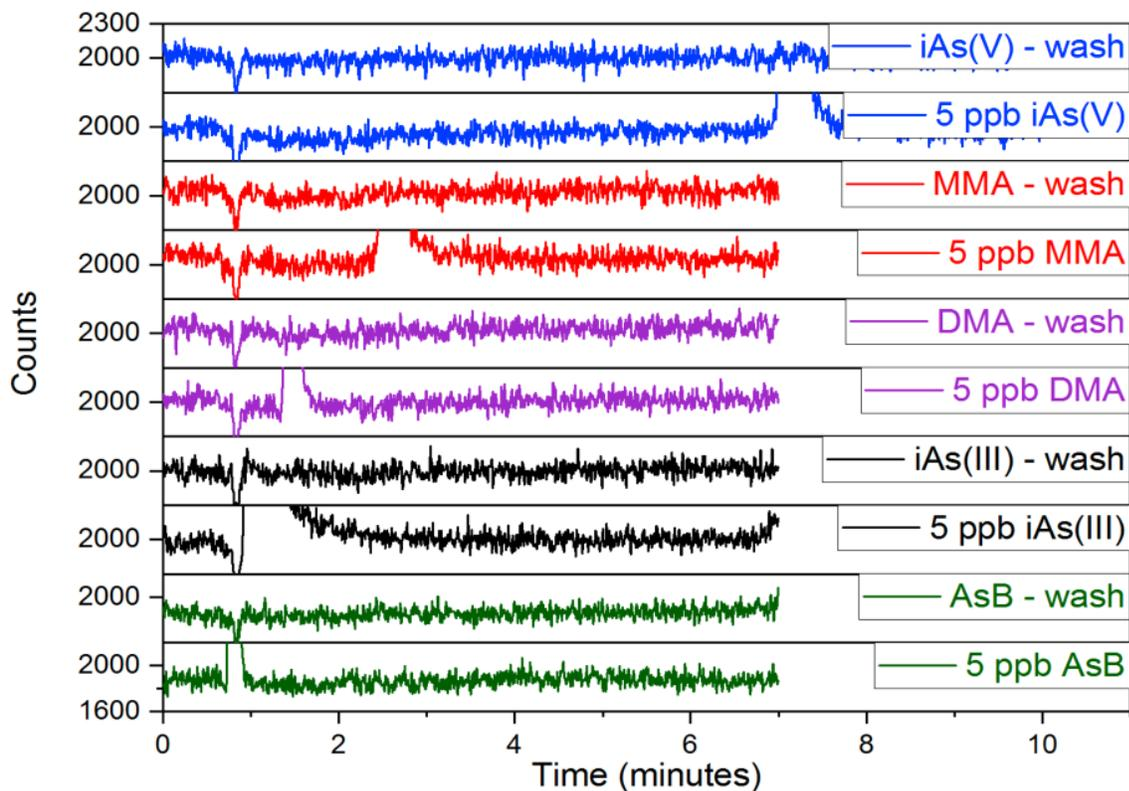
**Figure 2.9** Chromatogram showing runs of individual 5 µg/L As standards, and a run of blank water following each 5 µg/L (ppb) As run (zoomed in).
