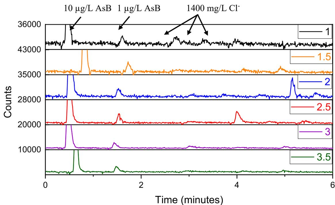
**Figure 2.6** Flow injection analysis (50  $\mu\text{L}$ ) of, in order of injection, 10  $\mu\text{g/L}$  AsB, 1  $\mu\text{g/L}$  AsB, and multiple injections of 1400  $\text{mg/L}$  chloride at various helium gas rates ranging from 1.00  $\text{mL/min}$  to 3.50  $\text{mL/min}$ . The nebulizer speed was kept at 0.5  $\text{rpm/min}$ . A volume of 50  $\mu\text{L}$  of each solution was manually injected (the chloride solution was injected multiple times in each run).
