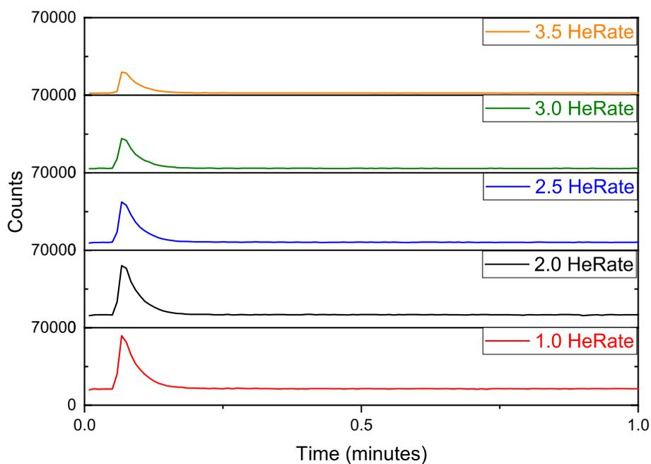
**Figure 2.7 Injection of 50 µg/L Mixed As standard (10 µg/L each of AsB, iAs<sup>III</sup>, DMA, MMA, and iAs<sup>V</sup>) at helium gas rates ranging from 1.00 mL/min to 3.50 mL/min.**
