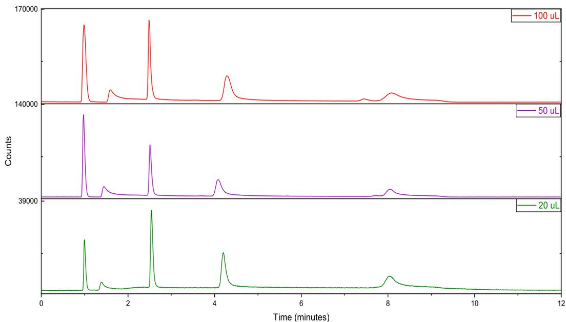
**Figure 2.4** 10 µg/L mixed standards of AsB, iAs<sup>III</sup>, DMA, MMA, and iAs<sup>V</sup>, injected with volumes of 20 µL, 50 µL, and 100 µL.
