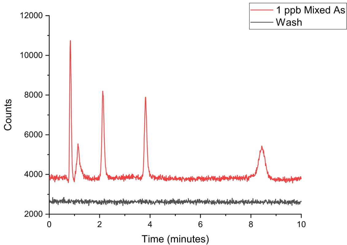
**Figure 2.10 Chromatogram showing a run of 1  $\mu\text{g/L}$  (ppb) mixed As, and a run of the wash collected after the 1  $\mu\text{g/L}$  Mixed As run was completed.**
