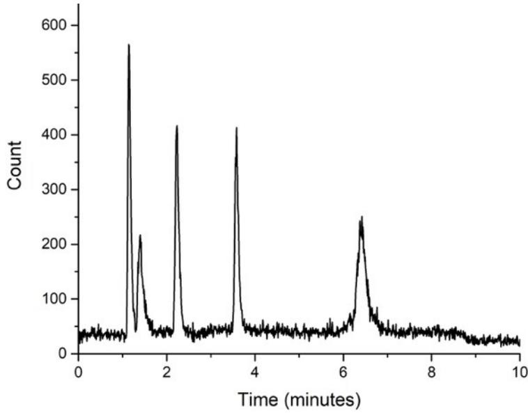
**Figure 2.16** Detection limit of  $iAs^{III}$  using  $1 \mu\text{g/L}$  arsenic standard
