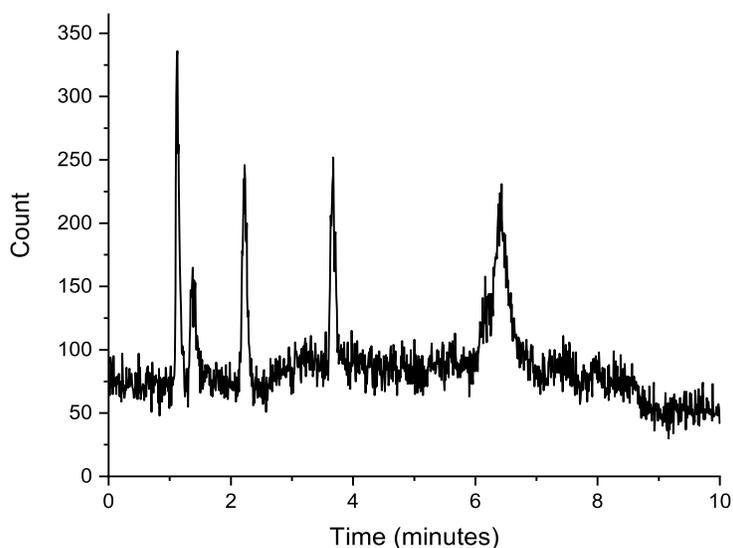
**Figure 2.15** Detection limits of AsB, DMA, MMA, and iAs<sup>V</sup> using 0.05  $\mu\text{g/L}$  arsenic standard
