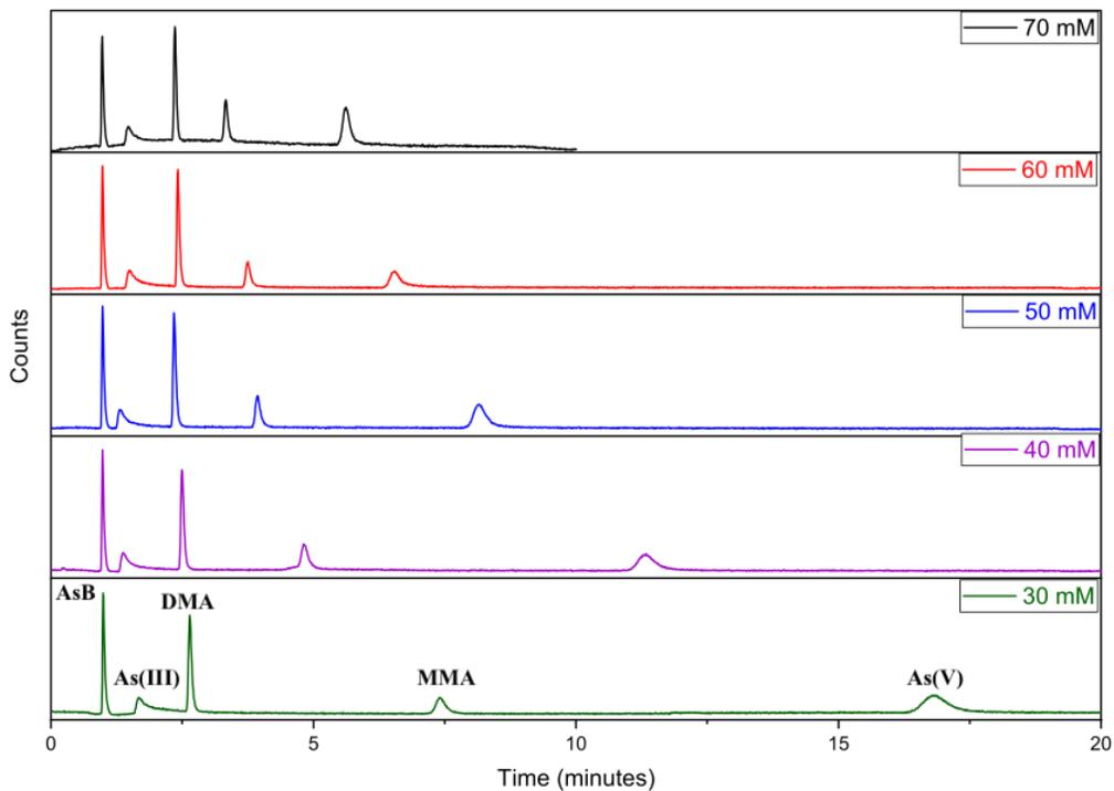
**Figure 2.2 Separation of 10  $\mu\text{g/L}$  AsB,  $\text{iAs}^{\text{III}}$ , DMA, MMA, and  $\text{iAs}^{\text{V}}$  using different mobile phase (pH 8.5) ammonium bicarbonate concentrations (from 30 mM to 70 mM).**
