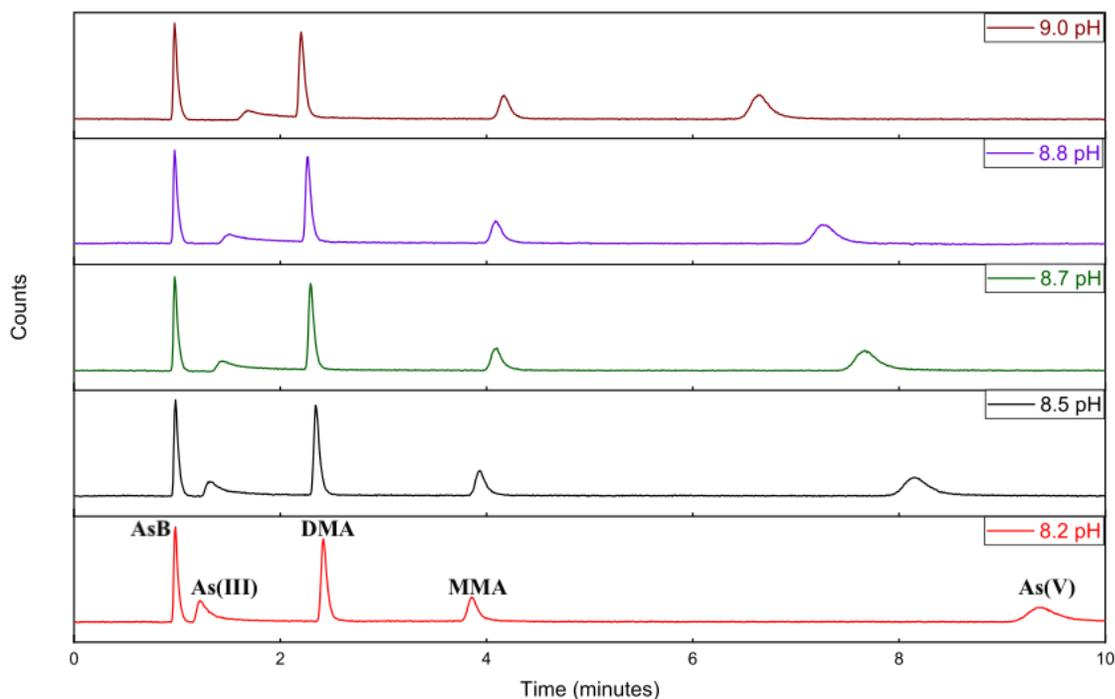
**Figure 2.3** Separation of 10  $\mu\text{g/L}$  AsB,  $\text{iAs}^{\text{III}}$ , DMA, MMA, and  $\text{iAs}^{\text{V}}$  using mobile phases (50 mM ammonium bicarbonate) of different pH values (from 8.2 to 9.0) using 10%  $\text{NH}_4\text{OH}$ .
