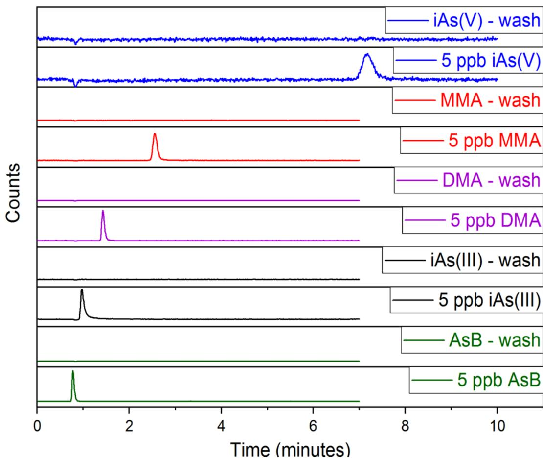
**Figure 2.8** Chromatogram showing runs of individual 5  $\mu\text{g/L}$  As standards, and a run of blank water following each 5  $\mu\text{g/L}$  (ppb) As run.
