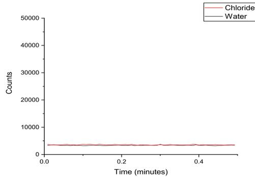
**Figure 2.5** Baselines of a pure 18.2 M $\Omega$ -cm water and a 1400 mg/L chloride solution through direct aspiration to ICPMS (no HPLC) at various helium gas flow rates ranging from 1.00 mL/min to 4.00 mL/min. The nebulizer pump speed was kept at 0.5 rpm/min.
