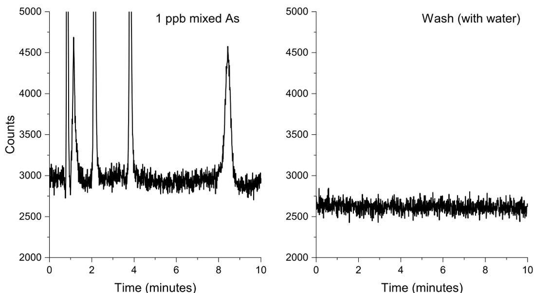
**Figure 2.11 Chromatogram showing a run of 1  $\mu\text{g/L}$  (ppb) mixed As, and a run of the wash collected after the 1  $\mu\text{g/L}$  Mixed As run was completed (zoomed in).**
