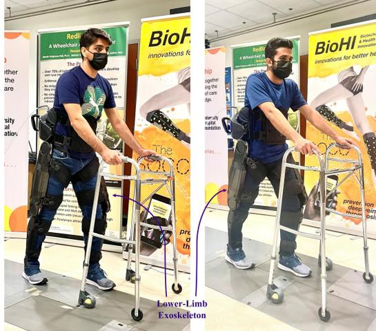
Figure 3.3: Indego lower-limb exoskeleton worn by two able-bodied users for over-ground walking: first participant (33 year-old) and second participant (27 year-old)
