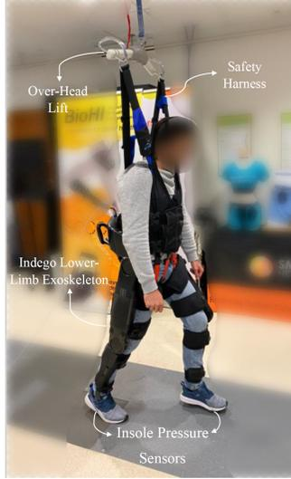
Figure 7.4: Experimental set-up: Indego lower-limb exoskeleton in a user study (having a safety harness) during over-ground walking
