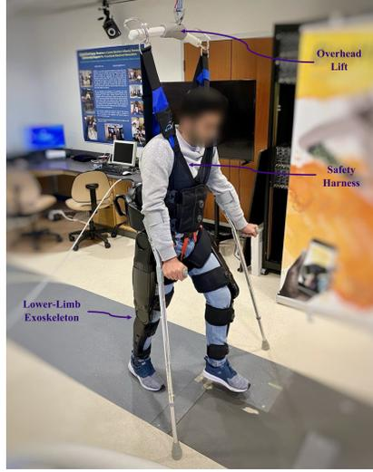
Figure 4.2: Indego lower-limb exoskeleton assisting a human user in overground walking with a safety harness
