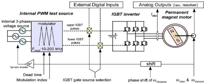
Fig. 5. PMSM drive model implemented on FPGA.
