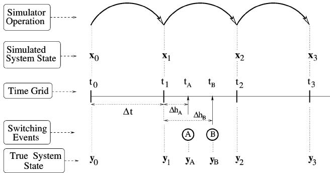
Fig. 2. Inter-step switching events in power-electronic system simulation.
