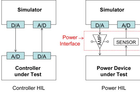
Fig. 1. Controller HIL simulation versus power HIL simulation.
