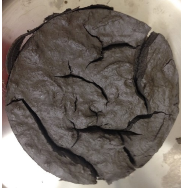
Figure 4.11 Cracks on filter cake at 600 kPa (4 kg/t Alcomer 7115 and 1 kg/t A3335).
