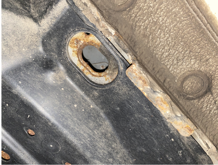
Figure 1.1: Example of metal corrosion phenomenon on the chassis of a car
