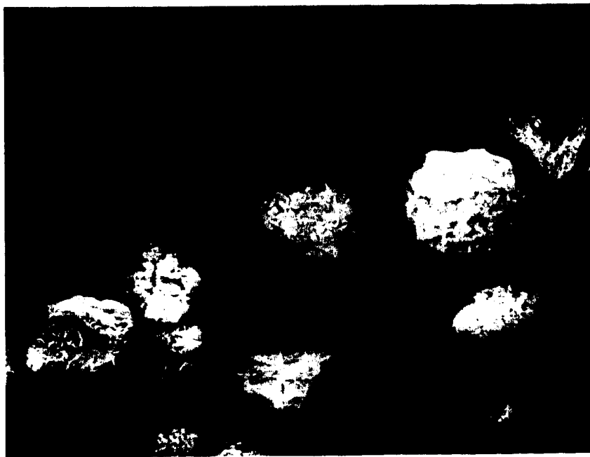
Figure 17. Electron Photomicrograph of Ash from 60 mesh Coke, 90X.
