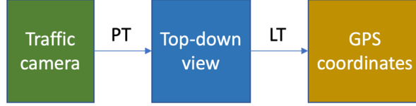
Figure 3.3: Method Used to Transform Pixel Coordinates to GPS Coordinates.
