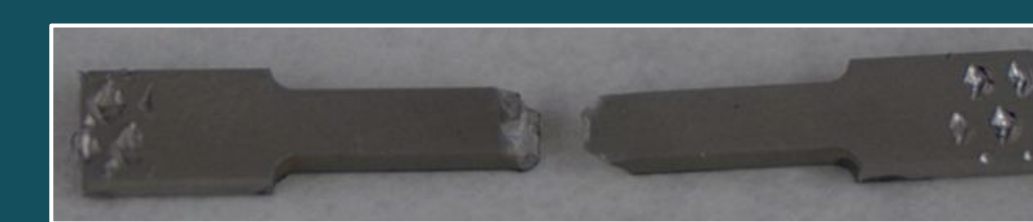
Fig. 7- Brittle fracture (Tensile testing result)
