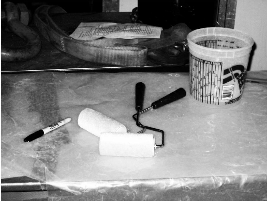
Figure 3-11 Polyurethane protected work surface.
