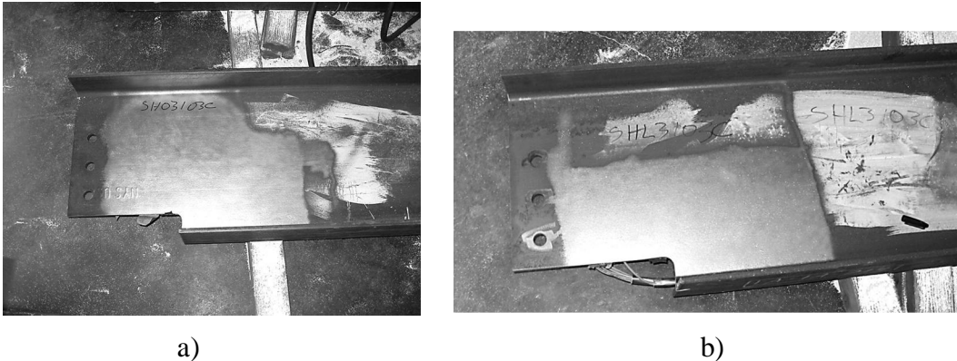
Figure 3-9 Beams prepared to white metal surface condition a) SHO3103C b) SHL3103C
