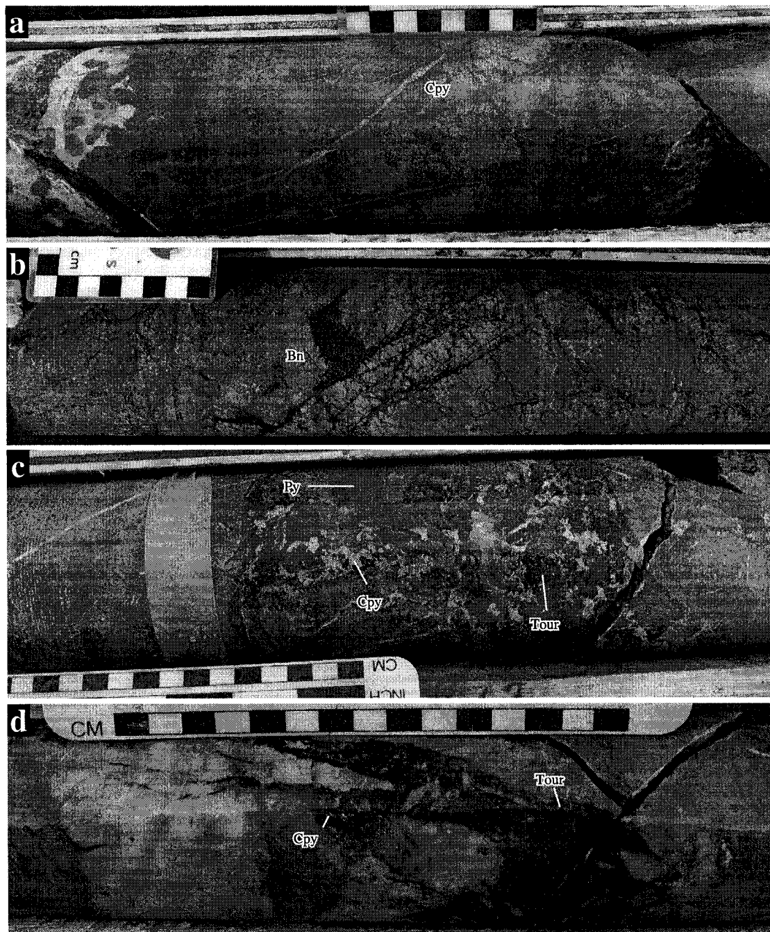
Figure 5.10 - (a) Chalcopyrite stringer with a sericite-chlorite alteration halo cross-cutting propylitic alteration in andesite. Drillhole 06CF258 at 222.8 m. (b) Bornite crackle breccia. Weak potassic vein-centric alteration has been overprinted by more pervasive sericite-chlorite alteration imparting a grey washed-out appearance to the volcanic rock. Drillhole 06CF254 at 81.1 m. (c) West Breccia zone mineralization. Hydrothermal breccia of sericite-chlorite altered volcanic rocks, cemented by tourmaline-quartz-carbonate with chalcopyrite and pyrite mineralization. Drillhole 05CF234 at 131.6 m. (d) Quartz-tourmaline vein with trace disseminated chalcopyrite. The vein locally brecciates the potassically altered volcanic host. The quartz portion of this vein does not contain any noticeable chalcopyrite mineralization. Drillhole 06CF277 at 156.1 m. Abbreviations: Bn = bornite, Cpy = chalcopyrite, Py = pyrite, Tour = tourmaline.
