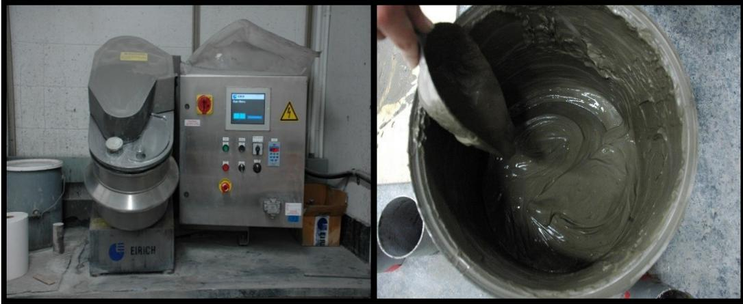
**Figure 6.1.** EIRICH high shear mixer (left) and the prepared cementitious paste (right)
