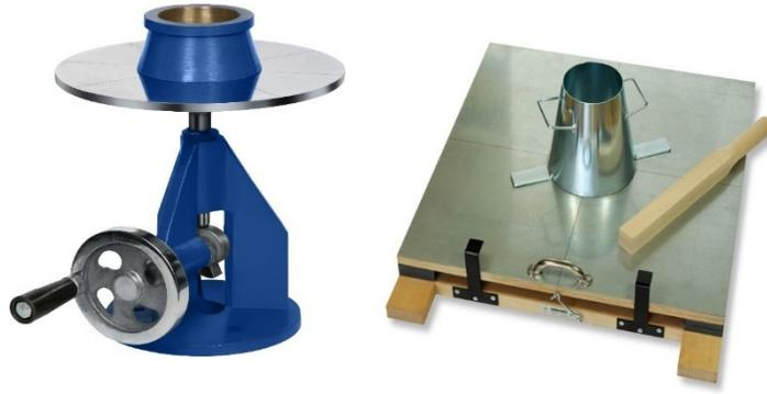
**Figure 3.8.** Flow table (left) and mini slump cone (right) employed to investigate the workability of prepared cement paste.
