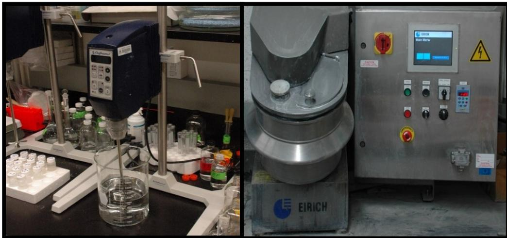
**Figure 4.1.** Mixers used to prepare bentonite/CNC suspensions (left) and oil well cement slurry (right)
