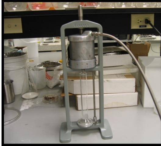
**Figure 3.9.** The static filtration test setup
