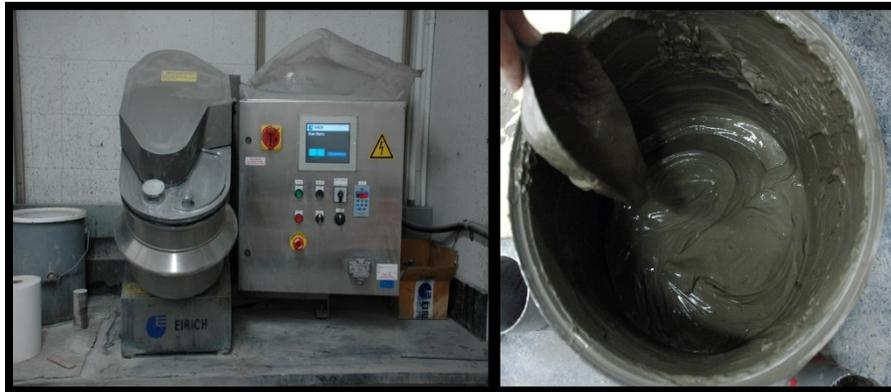
**Figure 3.5.** High shear mixer (left) and the prepared cementitious slurry samples (right)
