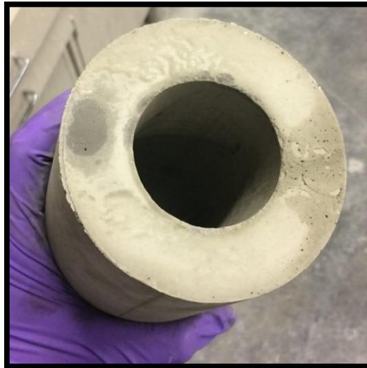
**Figure 6.2.** Hollow cylindrical samples prepared for the permeability test
