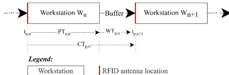
**Figure 5.5: Data collected from the RFID system**
