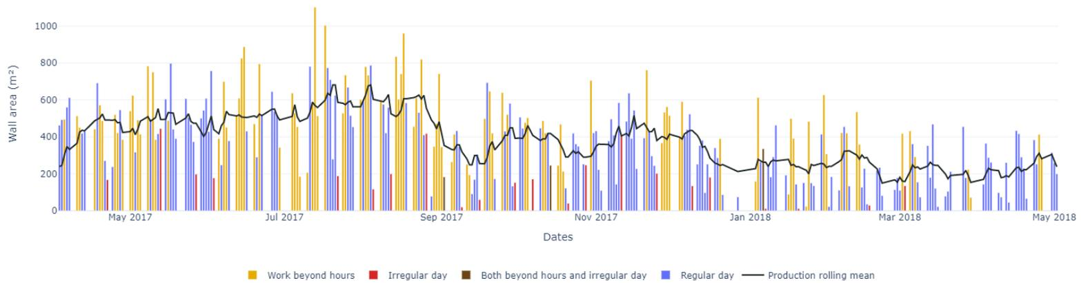
**Figure 5.3: Production rolling mean with a window of 14 days and daily production output according to approaches to maintain flexibility on sample data gathered on the shop floor**
