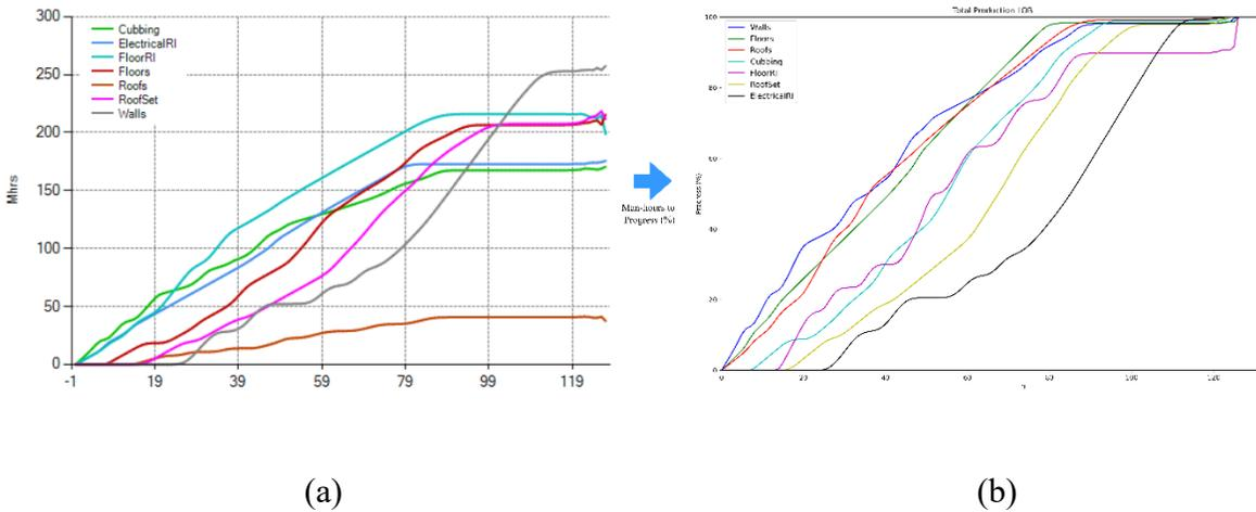
**Figure 6.3: Line of balance conversion from workstation man-hours to progress.**
