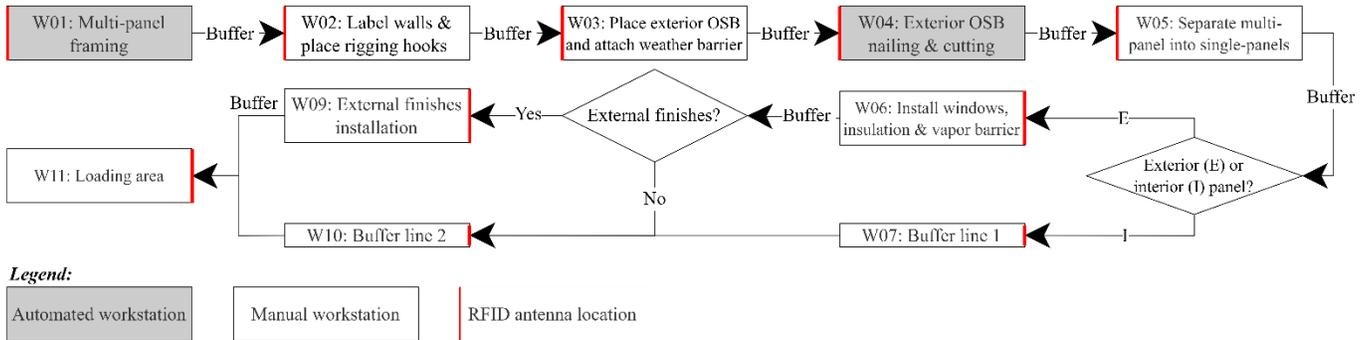
**Figure 5.1: Wall manufacturing tasks according to current workstations layout at the shop floor under study and locations of RFID antennas.**
