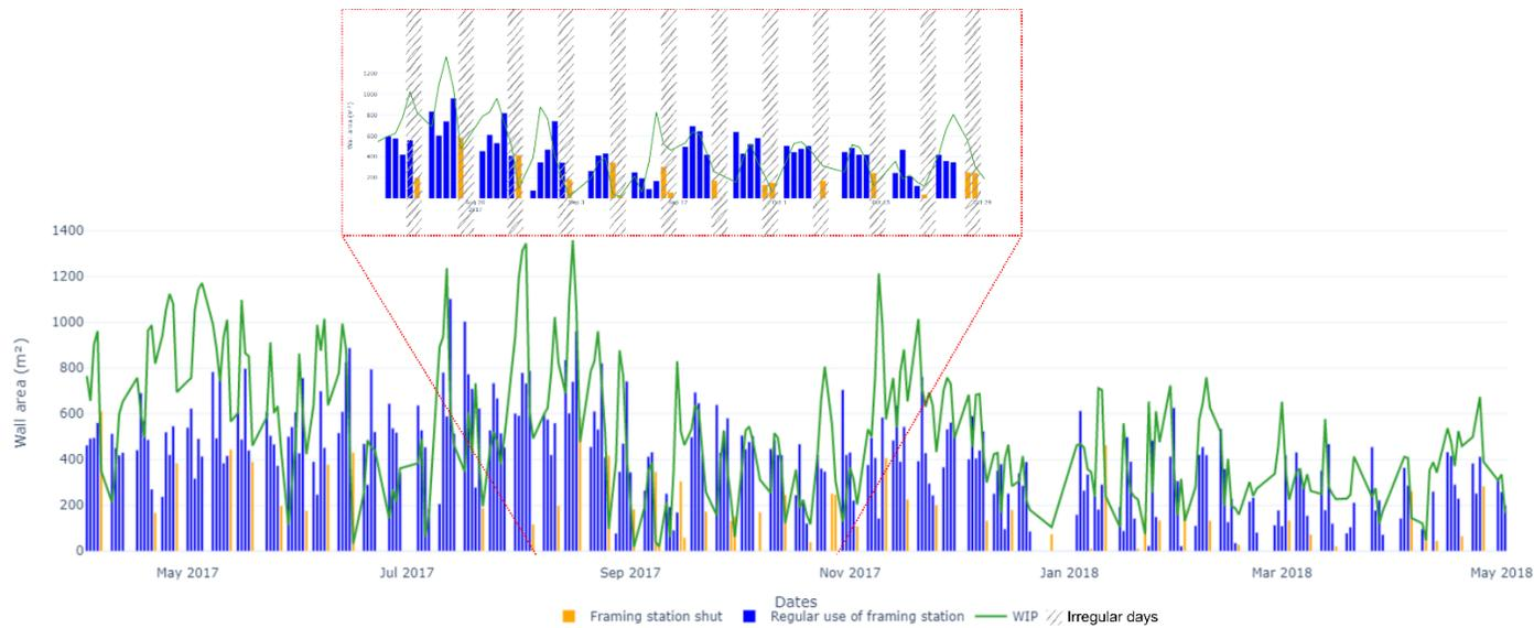
**3 Figure 5.4: Production output according to WIP, framing station status, and irregular days**
