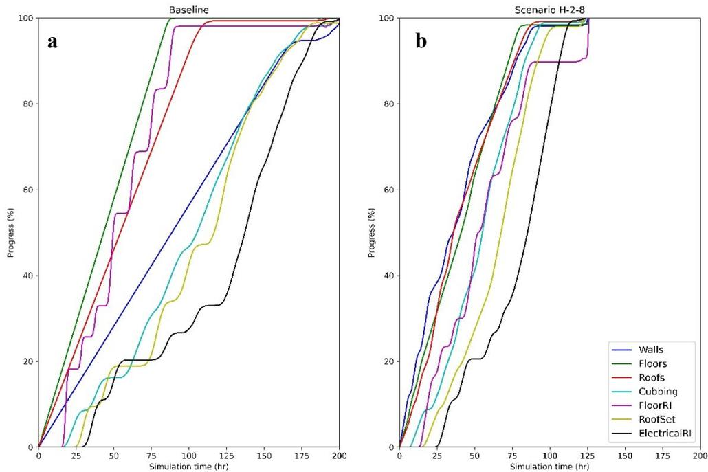
**Figure 6.8: Line of balance comparing the production between the baseline and scenario HB-2-8, respectively.**
