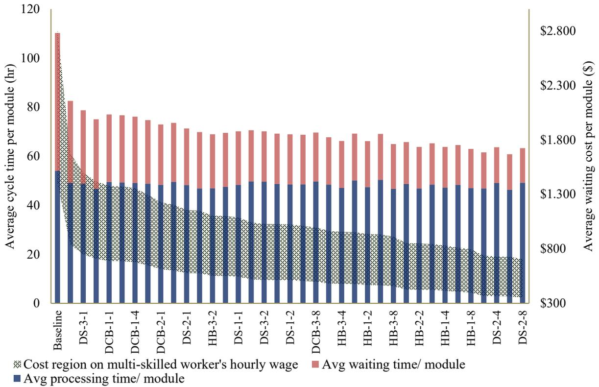
**Figure 6.6: Production efficiency assessment and average waiting cost per module.**
