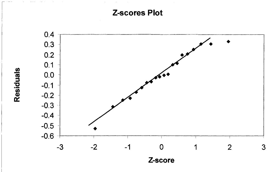
Figure C1- Normal probability plot for ANOVA residuals of UV inactivation of fecal coliform with and without sample pre-treatment
