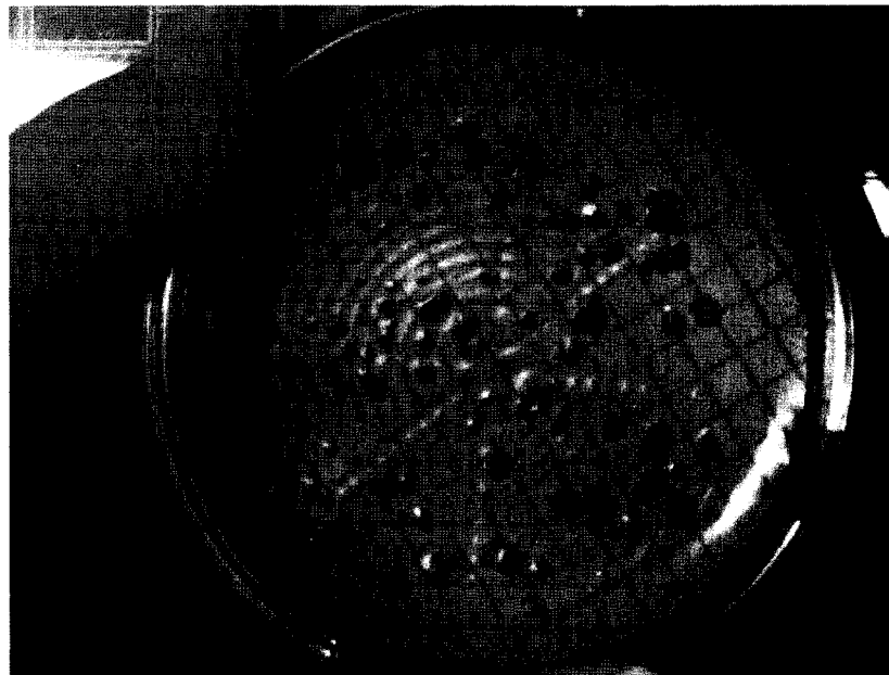
Figure 11: Fecal coliform colonies obtained from the Alberta Capital Region WWTP sample tested using the membrane filter technique
