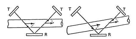
Angle Insensitivity of Transonic flowprobe: (T) = transducer; (R), reflector
