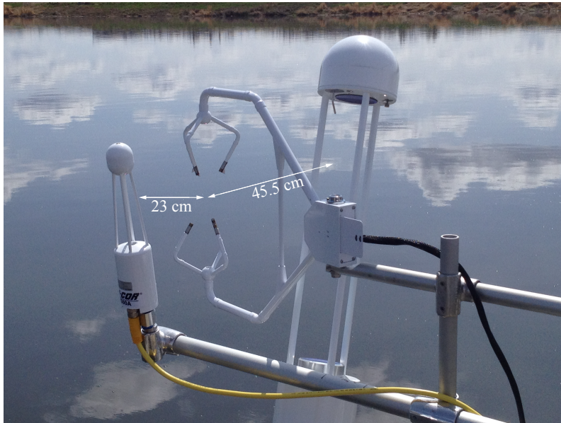
Figure 4.2: Eddy covariance instruments mounted on concrete jetty at biosolids lagoon field site: LI-7500A (left), CSAT3 sonic anemometer (centre), and LI-7700 (right). Separation distance between sensors is noted.
