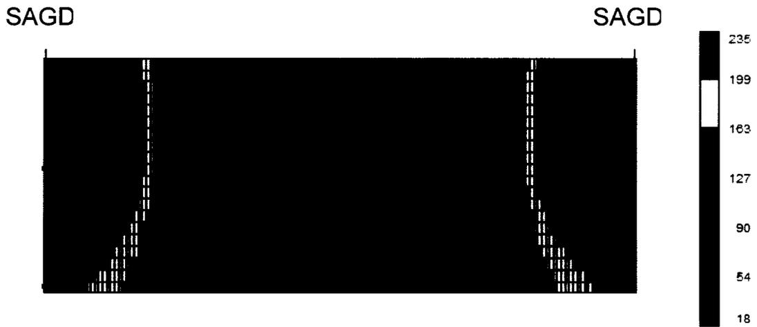
Figure 4.2a: SAGD steam chamber temperature profile after 5 years
