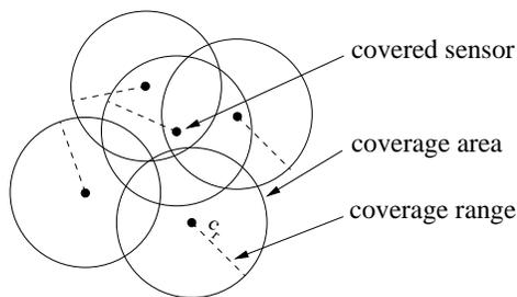
Figure 2: The coverage of sensors
