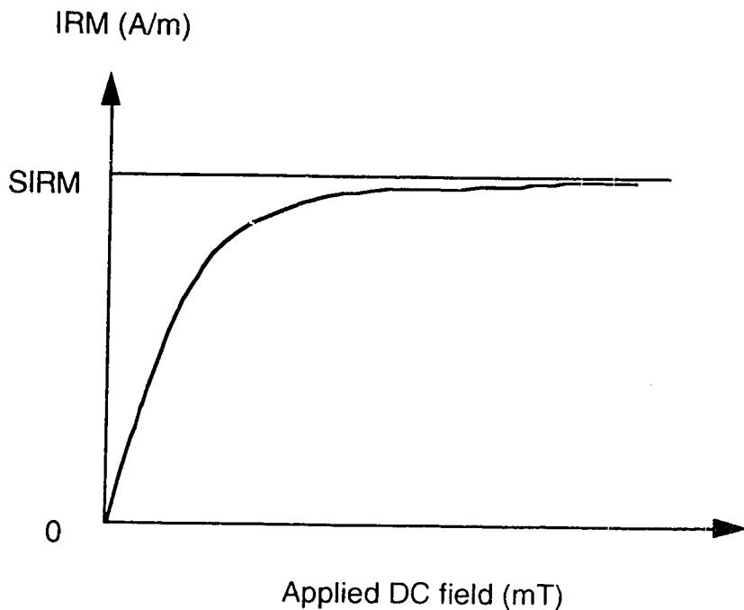
Figure 2.3. *IRM acquisition curve*
