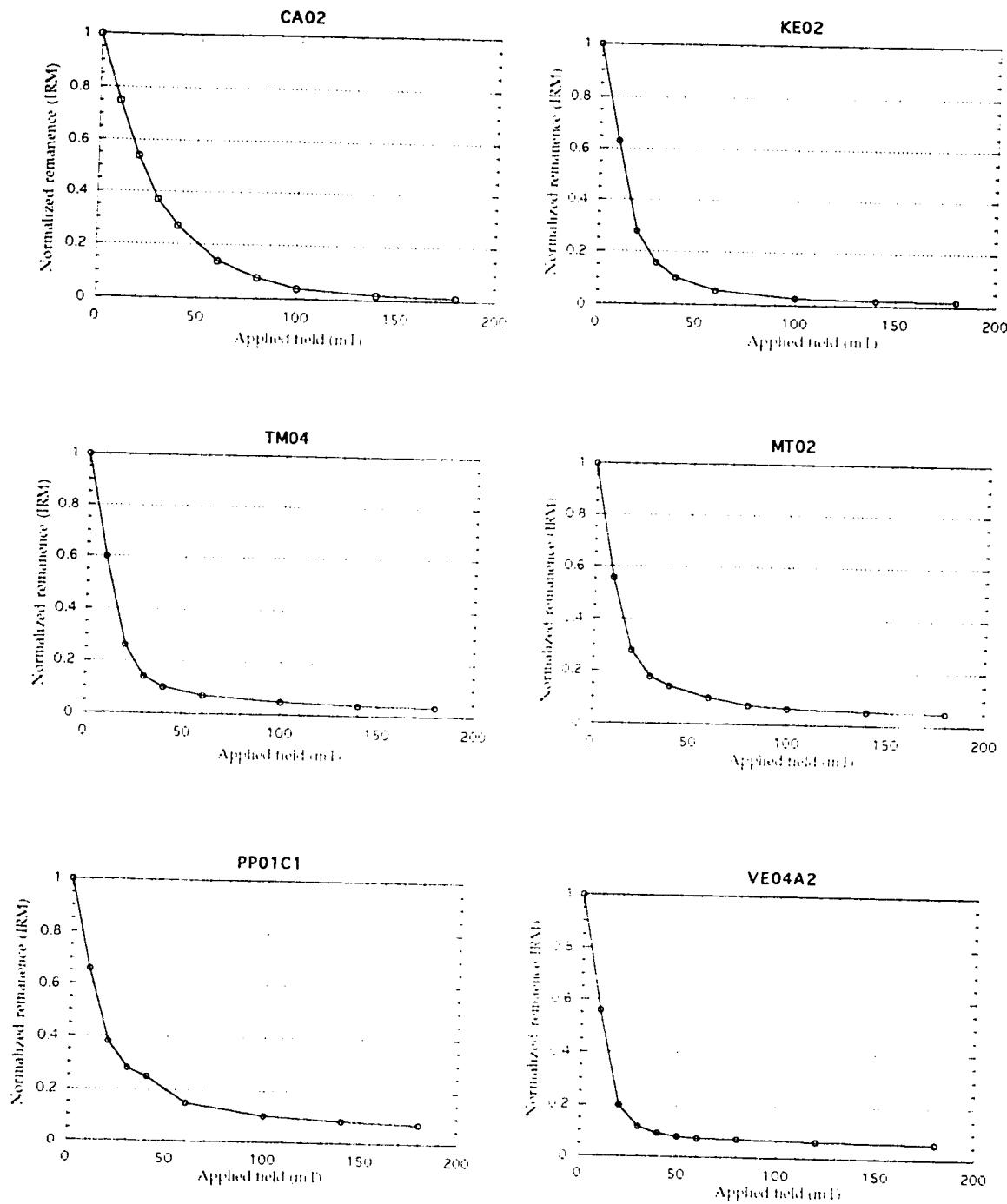
Figure 3.2.5b *AF demagnetisation of IRM of Italian samples*
