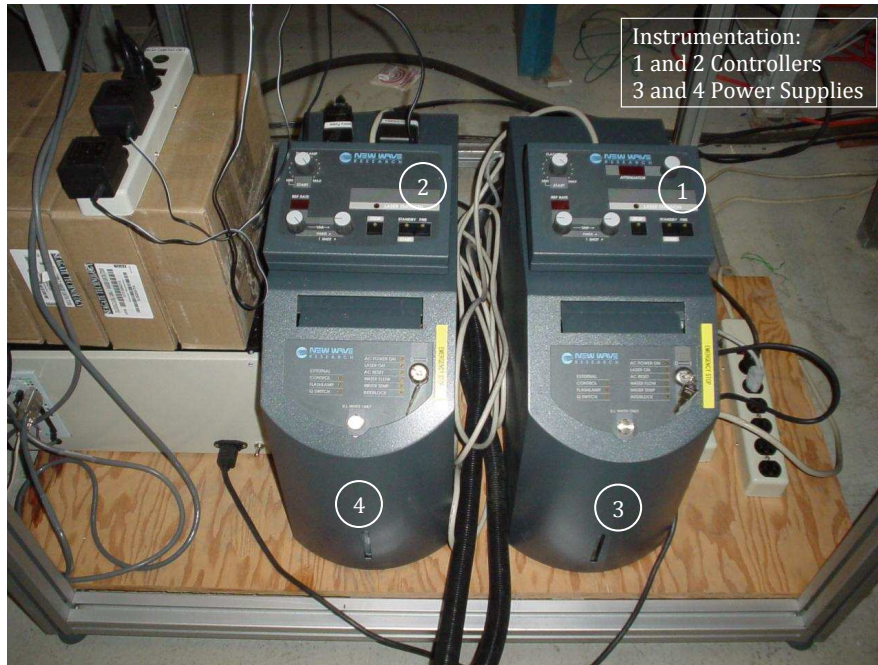
Figure 2.4: A photograph of Nd:YAG laser control panels and dual-power supply.
