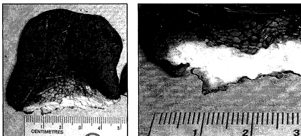
Figure 2.3-5. Polystyrene after 24-36 hrs in the beginning stages of the composting process.
