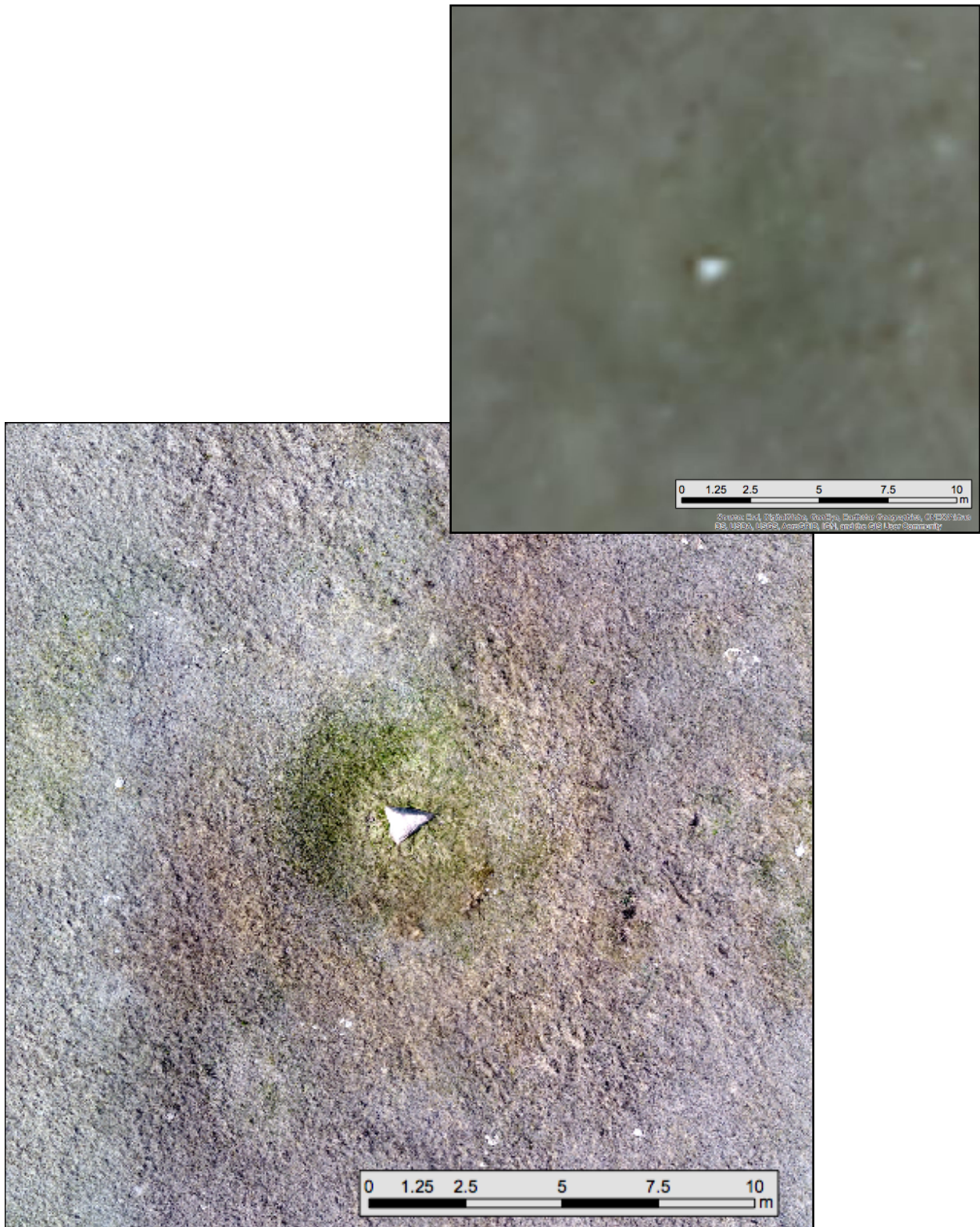
Figure 4.4: Satellite imagery (top) and drone image (bottom) of the rubbing stone showing the difference in the resolution of the imagery data. Note that the drone data shows the depression surrounding the stone and the vegetation difference.
