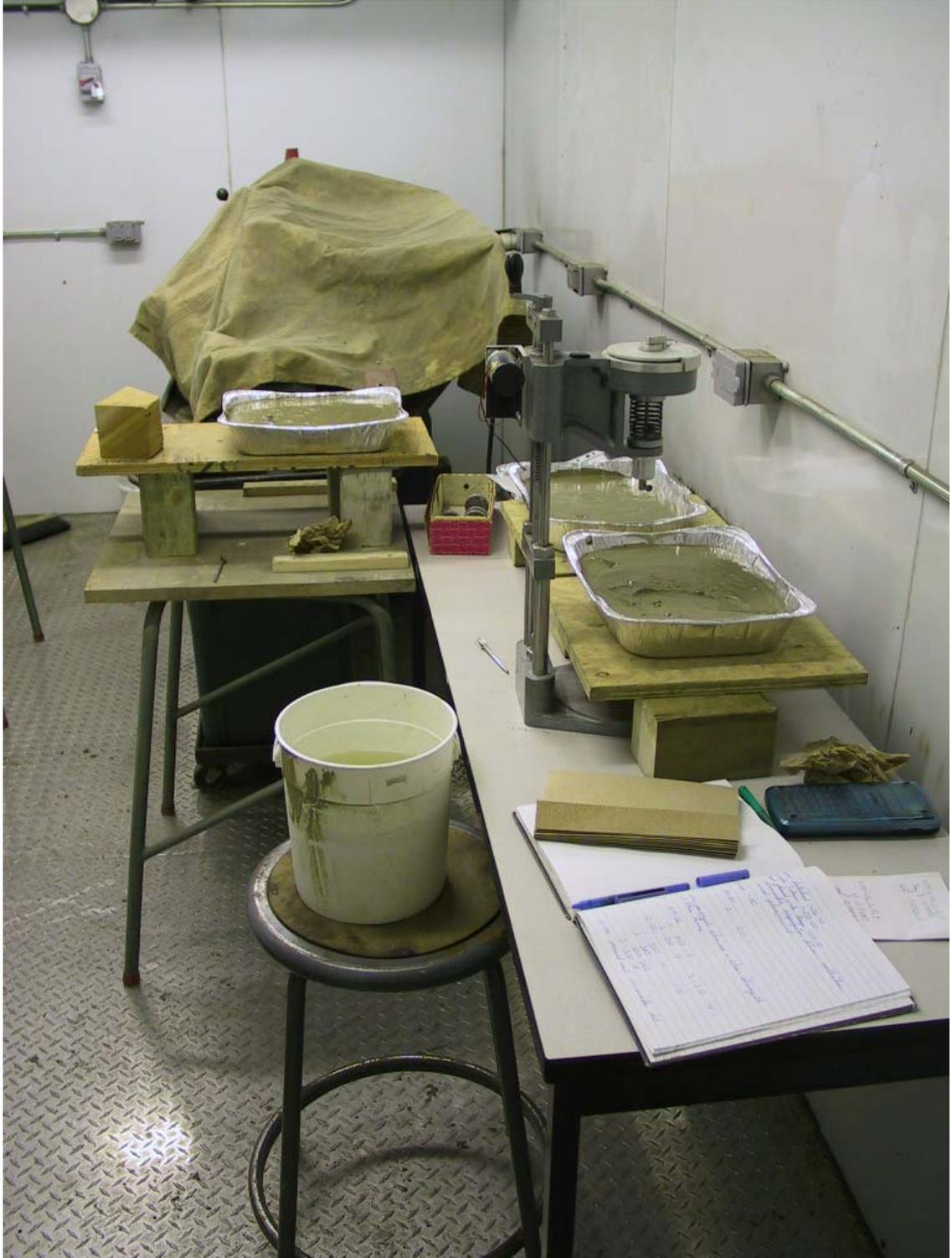
Figure 4-49 Set-up for testing of grout.
