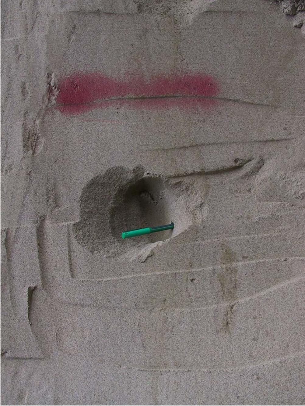
Figure 3-9 Enlargement of a siltier zone within the Outwash Sands and Silts from Figure 3-6 (elevation of ~661.5m, ~3m east of West Wall).
