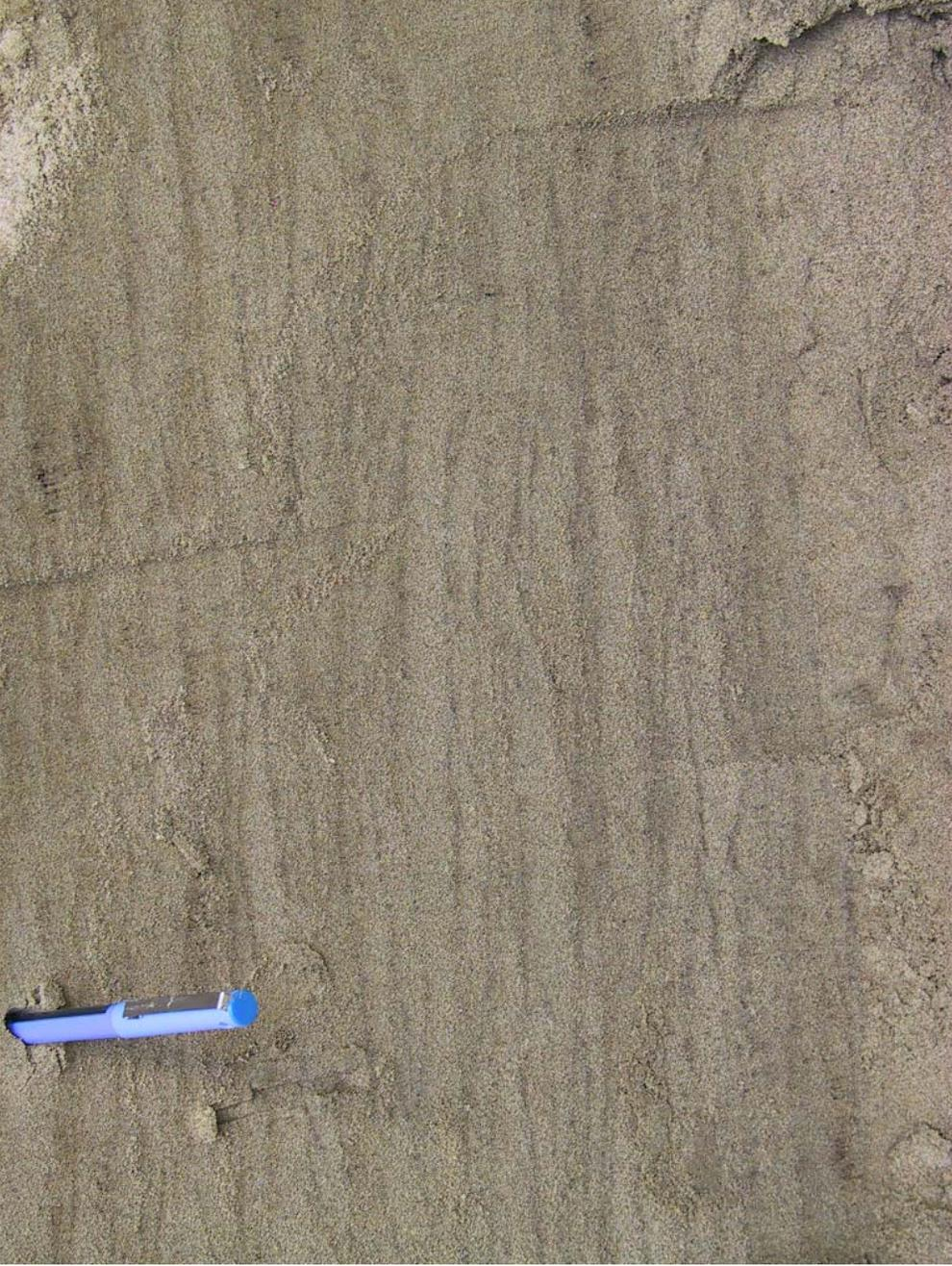
Figure 3-10 Enlargement of sand with silt inter-bedding visible in Figure 3-7 (elevation ~660.5, ~1.3m west of East Wall).
