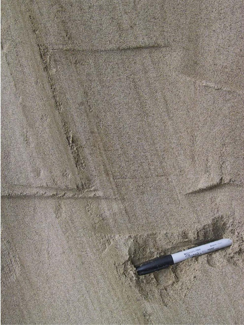
Figure 3-8 Enlargement of silt stringers within sand visible in Figure 3-6 (elevation ~661.5m, ~1m east of West Wall).
