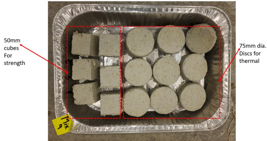
Figure 6.5: Hempcrete samples after demolding
