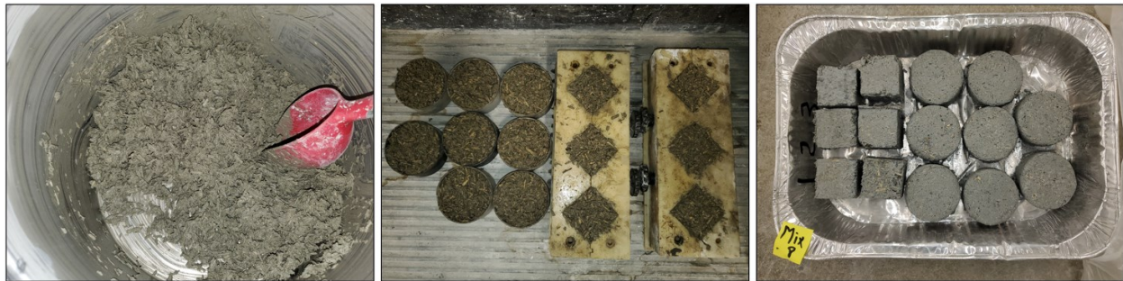
Figure 5.12: Mixing, casting, and demolding hempcrete samples for each mixture
