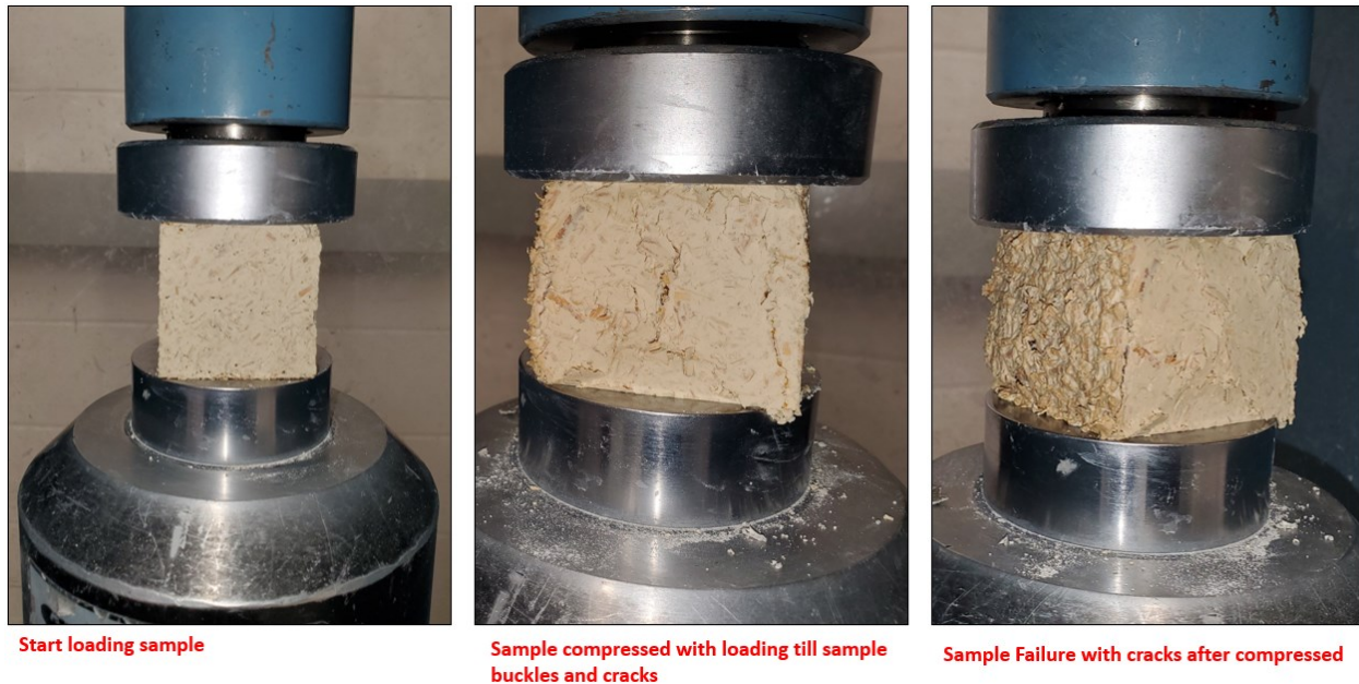
Figure 3.22: Compression test for a typical hempcrete sample showing failure mode (buckles and cracks)
