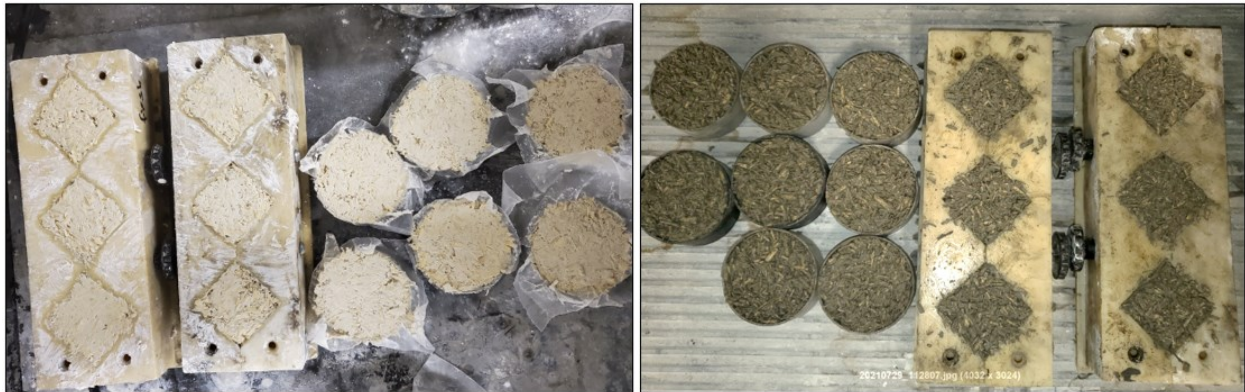
Figure 3.8: A typical freshly cast hemp concrete for lime and cement
