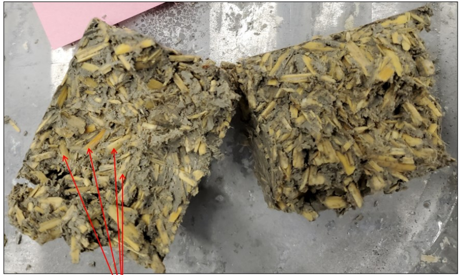
Failure at interface zone between hemp and binder for wet sample
