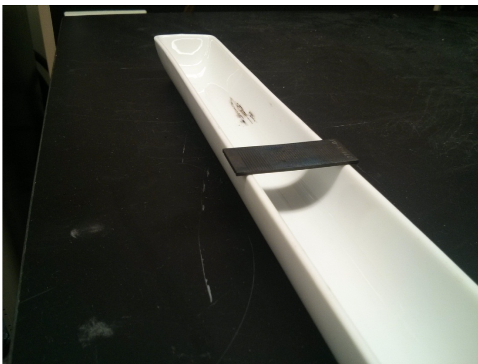
Figure 3.7 a,b a) (top) Reactor placed on the edges of the ceramic holder; b) (bottom) Reactor placed on the bottom surface of the ceramic holder
