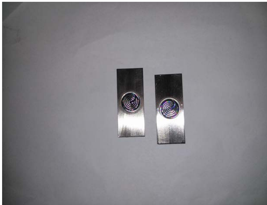
Figure 3.4 a, b a) (top) Diagram of Reactor I made of Iron/Nickel Alloy (Alloy 52) with a well for mixtures of reacting liquid and solid coke particles. The well depths were 0.6 mm, 1.2 mm or 2 mm, and the well diameter was 15 mm in all cases; b) (bottom) Top view of Reactor I.
