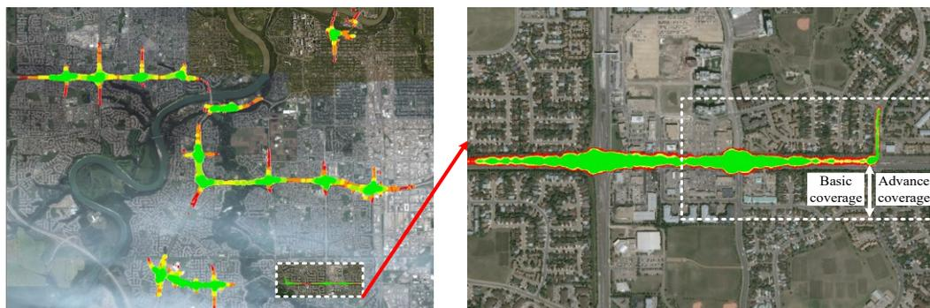
(a) RSE communication coverage of the ACTIVE CV testbed except for the South Campus area
