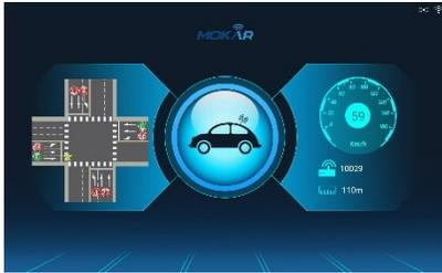
(d) SPaT, vehicle motion, and map information demonstrated by an illustrative interface prototype
