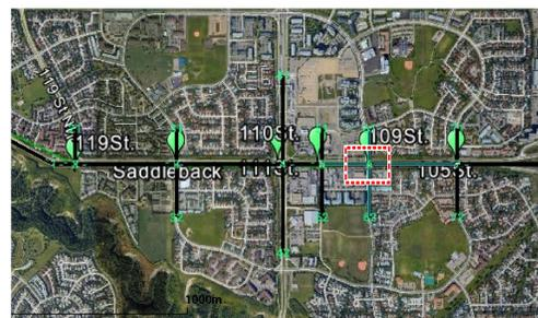
(b) RSE locations (green pins), the geometry (background picture), target intersection (dashed box), and a network representation (black lines) in SUMO traffic simulator
