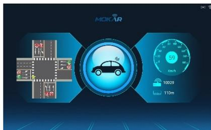
(b) SPaT, vehicle motion, and map information demonstrated by an illustrative interface prototype
