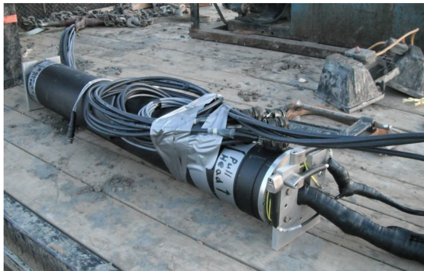
Figure 5.3. Watertight container hosting strain recording instrumentation
