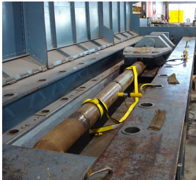
Figure B.1. Axial Strain Gauge Testing Procedure
