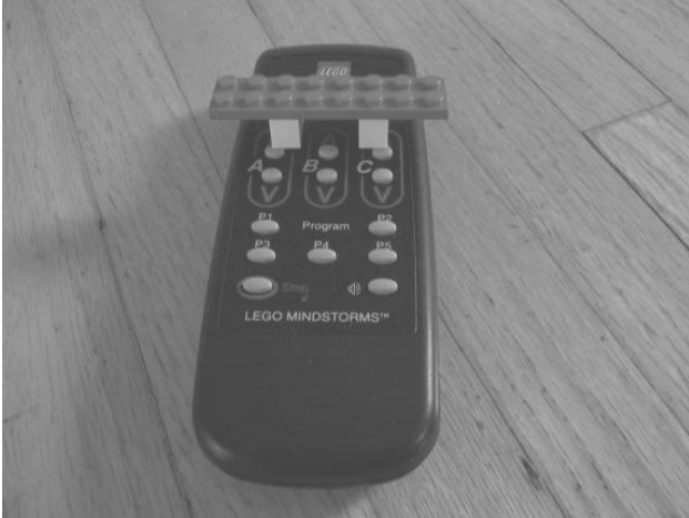
Figure 7: A Lego block device which ensures that the left and right motor buttons are pressed at once to obtain straight forward movement.
