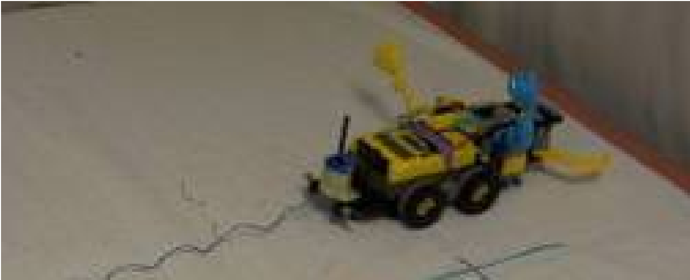
Figure 4: Robot with spindle to hold spool of string
