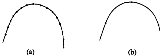
Figure 3.5: A snake discretized with different scales: it is considered (a) smooth using a small scale; (b) not smooth using a larger one.
