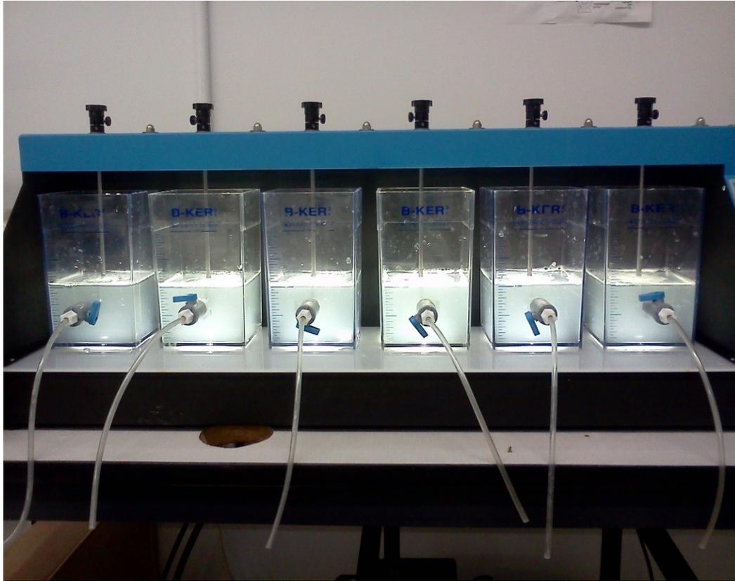
**Figure 3-4** Jar test unit with coagulated OSPW.
