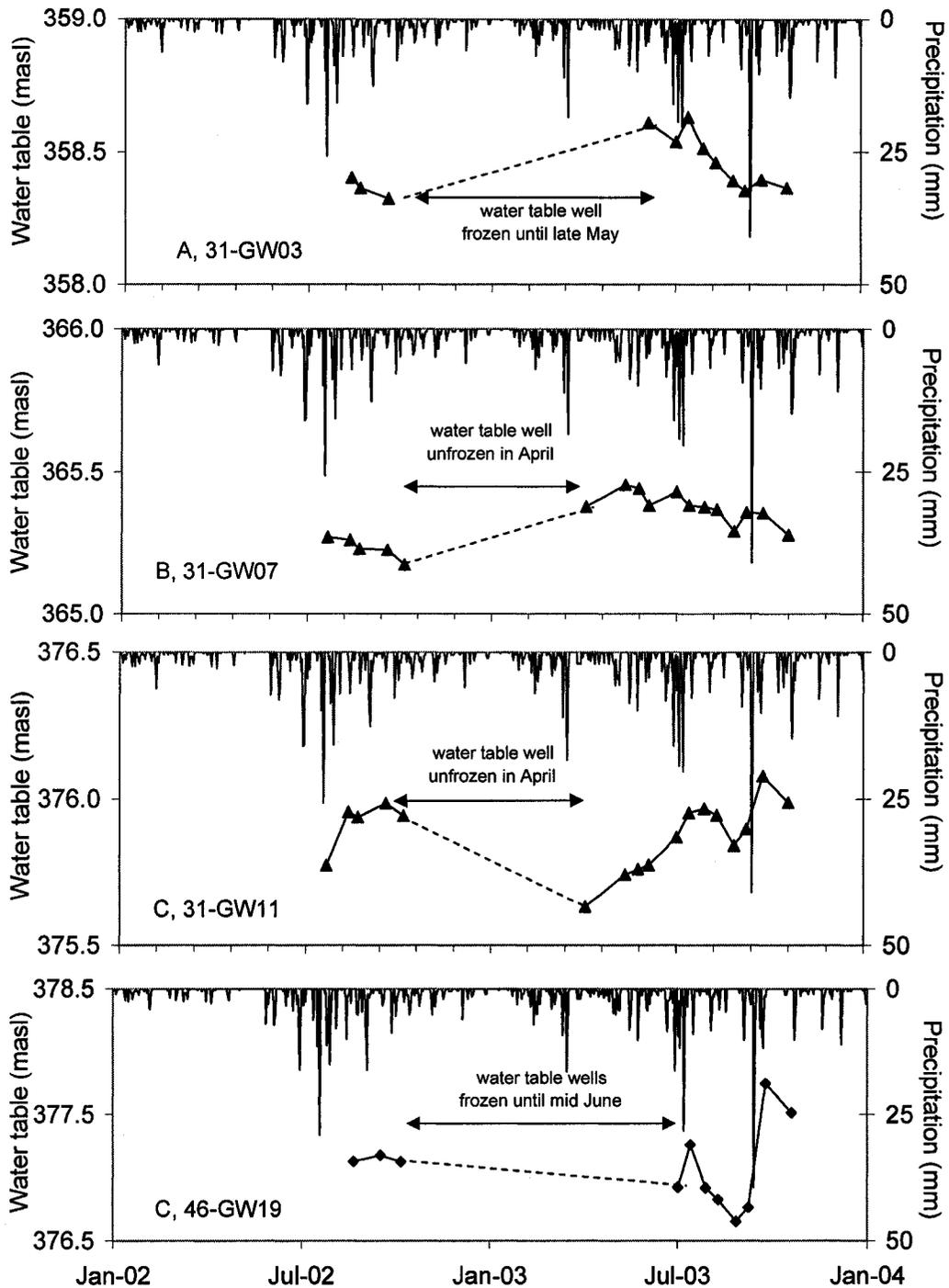
Figure 2-5. Seasonal water table response at the crests of Bench A (GW03), Bench B (GW07) and Bench C (GW11) on Transect 31 and Bench C (GW19) on Transect 46. Rain data from SWSS plus snow data from Ft McMurray Airport shown across the top axis (Okane, 2004; Environment Canada, 2004). Note change in vertical scale for Transect 46.
