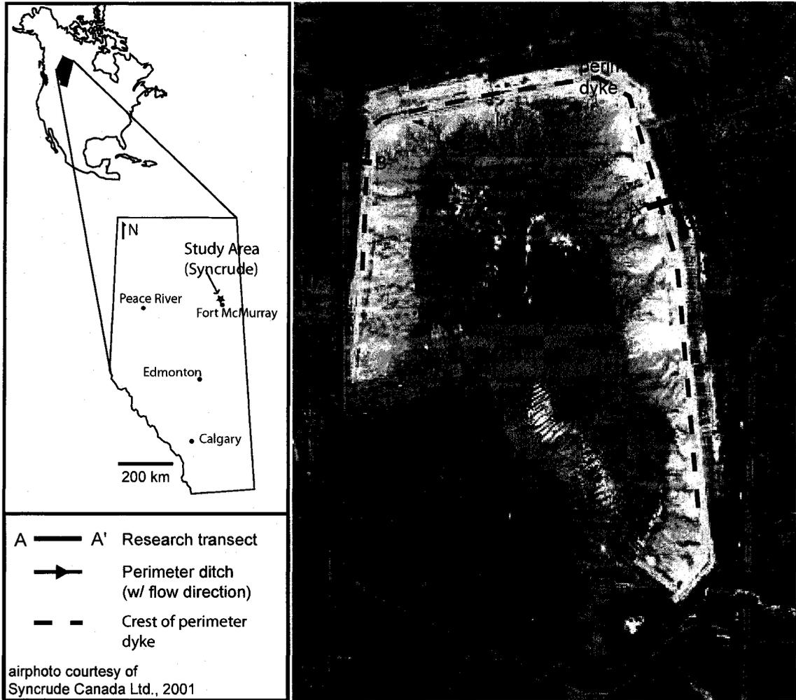
Figure 2-1. Research Transects 31(A - A') and 46 (B - B') at the Southwest Sand Storage Facility. Darker areas on the perimeter dyke indicate reclaimed areas in 2001. Insets show locations within Alberta and North America (top left).
