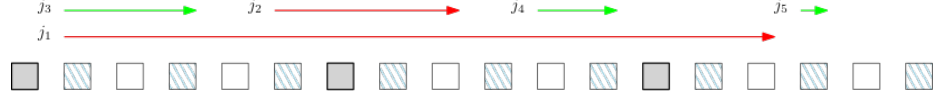
Figure 3.2: In this example, h = 3 , the dark squares represent the terminal machines in the first layer, which partition the machines into 3 segments. The squares with crossed lines represent the second layer terminal machines. The corresponding groups of jobs are defined as G_1 = \{j_1, j_2\} and G_2 = \{j_3, j_4, j_5\} .
