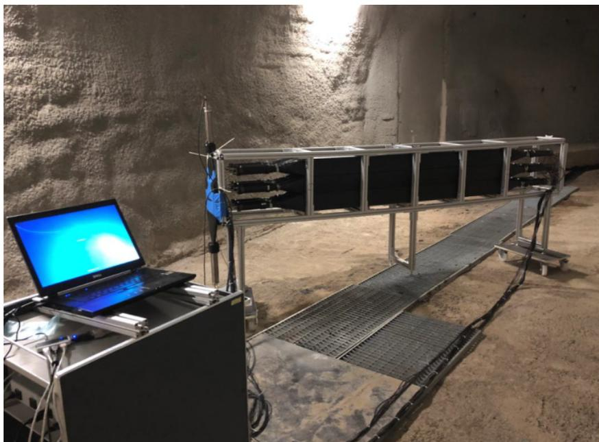
FIGURE 3.6. A digital photograph of the MAPP-mCP prototype detector deployed in the UGC1 gallery during Run-2. The readout electronics are also shown in the image.
