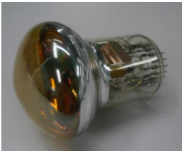
FIGURE 3.11. Photograph of an HZC Photonics model XP72B20 PMTs used in the MAPP-mCP detector.
