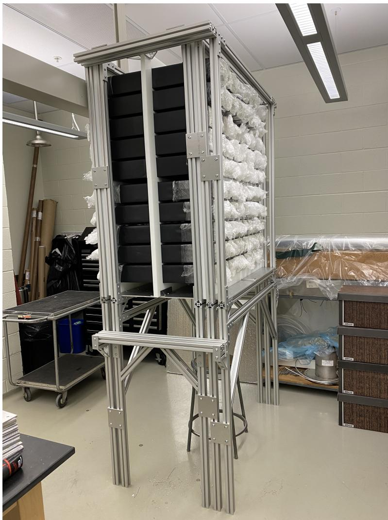
FIGURE 3.10. A digital photograph of one of the four collinear sections of the MAPP-mCP subdetector assembled with the full support structures and 100 scintillator units, demonstrating the successful load test.
