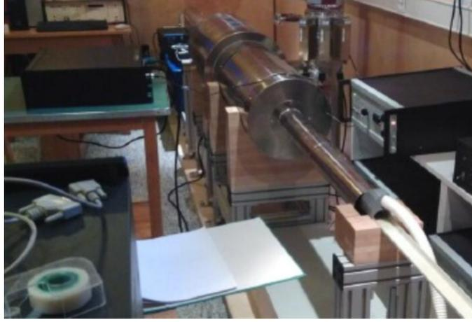
FIGURE 2.11. A photograph of the SQUID magnetometer from the ETH Zurich Laboratory of Neutral Magnetism, used to scan exposed MoEDAL MMT samples.
