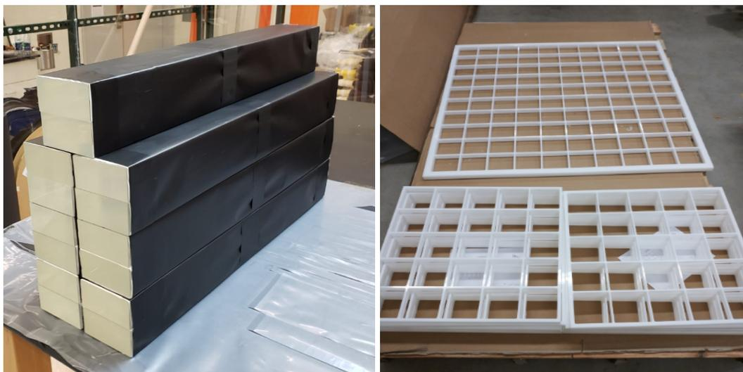
FIGURE 3.9. A stack of fully wrapped and prepared scintillator bars for the MAPP-mCP detector, and their polyethylene support frames.
