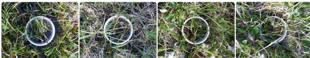
**Figure A1.3** Photos of collars used to measure dark soil respiration using the LI-6400. Vegetated and unvegetated soils at the polar semidesert and soils at the wetland are shown. Collars used from 2010–12 at both sites are shown only.
