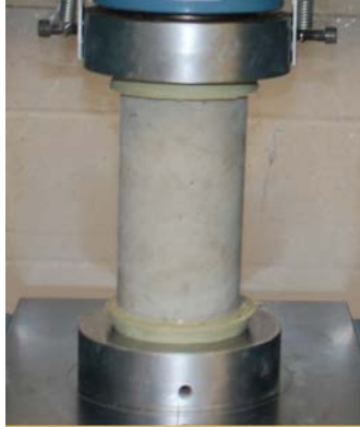
Figure A-10: Typical Compression Test of Concrete Cylinder.
