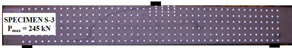
d) Crack Patterns after Failure
