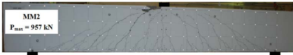
b) Crack Patterns after Failure
