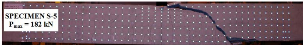
d) Crack Patterns after Failure
