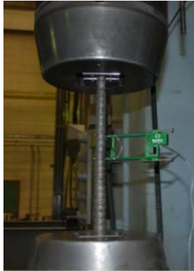
Figure A-11: Typical Tension Coupon Test of Steel Rebars.
