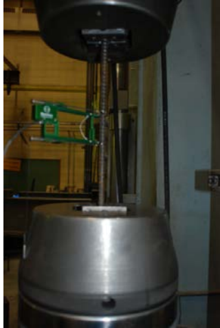
Figure A-2: Typical Tension Coupon Test of ASTM A1035 Steel Rebars.
