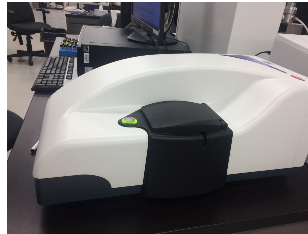
Figure 2.0: Zetasizer Nano-ZS used for measuring nanoparticle size
