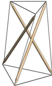
**Figure 2-11. One-stage tensegrity prism (simplest form of spatial tensegrities)**
