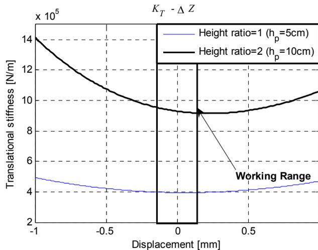
Figure 4-15. Effect of height ratio on translational TPS
