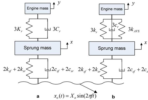
**Figure 3-8 Quarter model of a passenger car with a. the equivalent passive mount b. The VSM**
