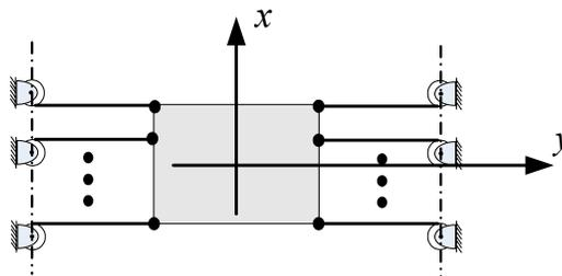
**Figure 3-4 A kinematically singular prestressable mechanism with four FOIM ( four singular directions).**
