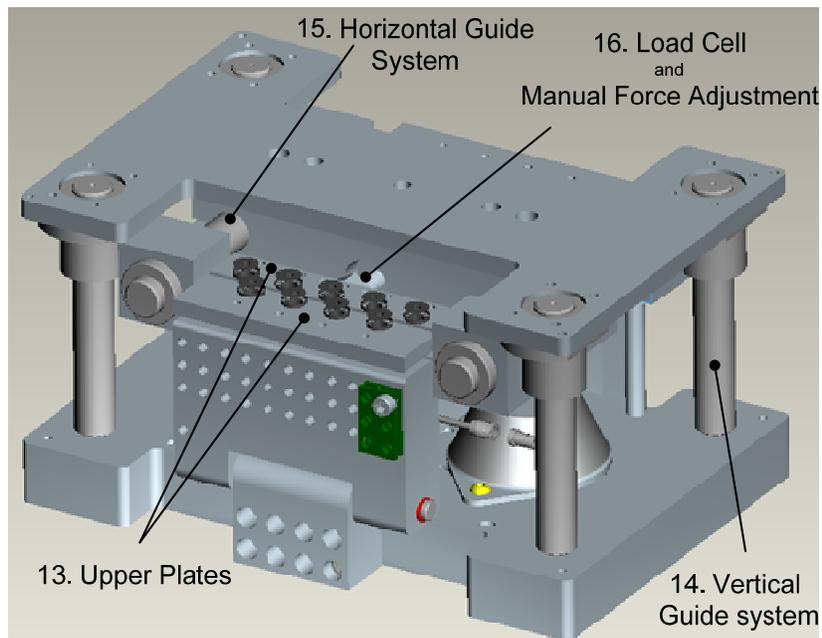
Figure 5-3 .Solid model of the VSM
