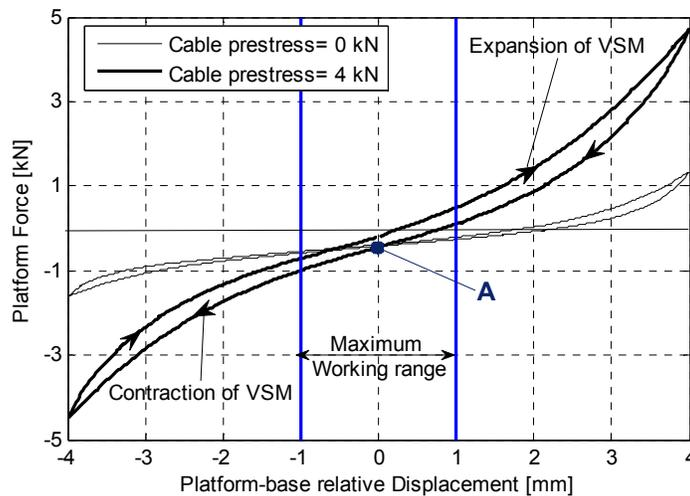
**Figure 5-15. Static test of the VSM with cable (VSM-C)**
