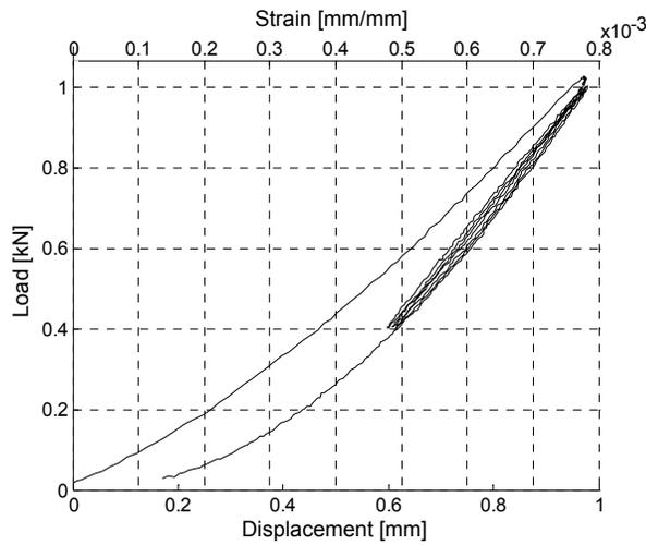
**Figure 5-6. Load – Strain and Load-displacement of the cable (Table 5-2) used in VSM**
