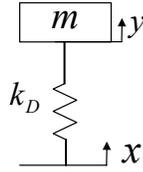
**Figure 5-24. Model of the VSM used for predicting the transmissibility of the VSM-C**
