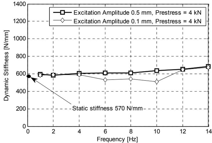
**Figure 5-22. Dynamic stiffness of the active VSM-P, prestress equals 4 kN, tested in different excitation frequencies**
