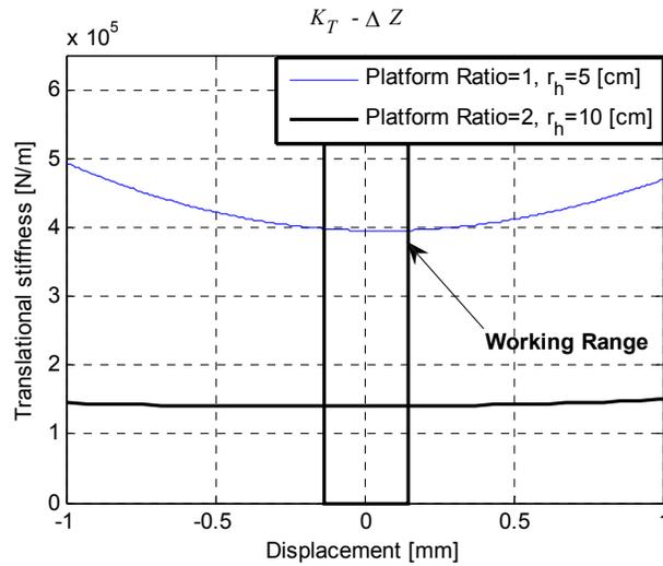
**Figure 4-16. Effects of platform ratio on translational TPS**
