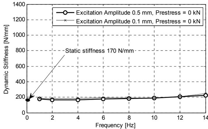
**Figure 5-21. Dynamic stiffness of the inactive VSM-P, prestress equals zero, tested in different excitation frequencies**
