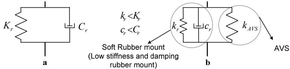
**Figure 3-6 a. Model of a typical passive mount b. Model of the VSM**
