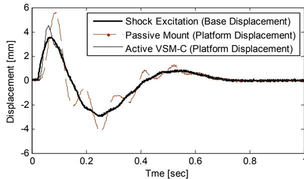
**Figure 5-31. Shock excitation at the base of the VSM-C and the resulted platform displacements**
