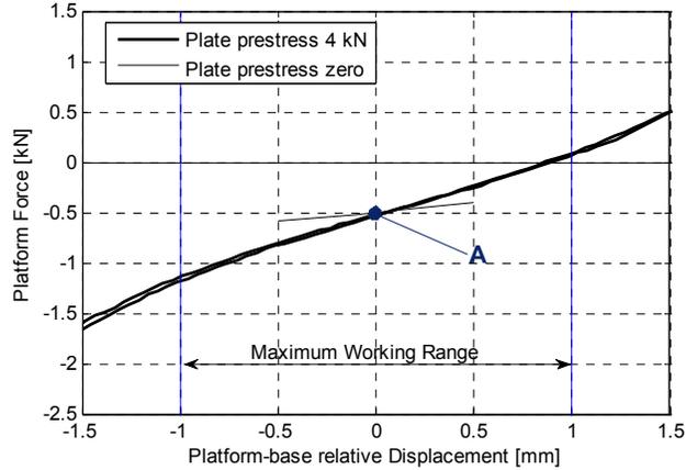
**Figure 5-16. Static test of the VSM with Plate (VSM-P)**
