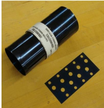
**Figure 5-8. Thin plate used in the VSM**
