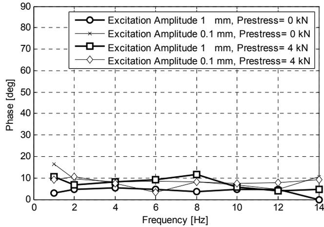
**Figure 5-20. Phase response of the inactive and the active VSM-C in different excitation frequencies**
