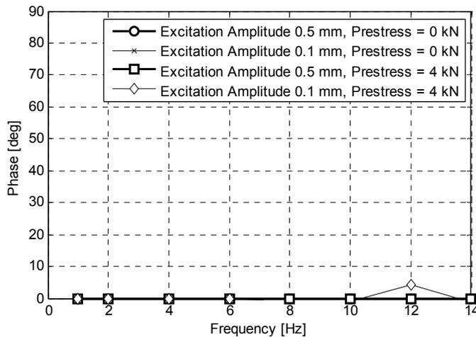
**Figure 5-23. Phase response of the inactive and the active VSM-P in different excitation frequencies**
