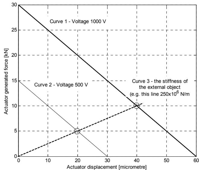
**Figure 5-10. Force-displacement characteristics of the piezo actuator**
