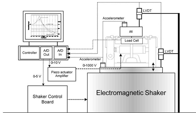
Figure 5-26. Shaker table set-up
