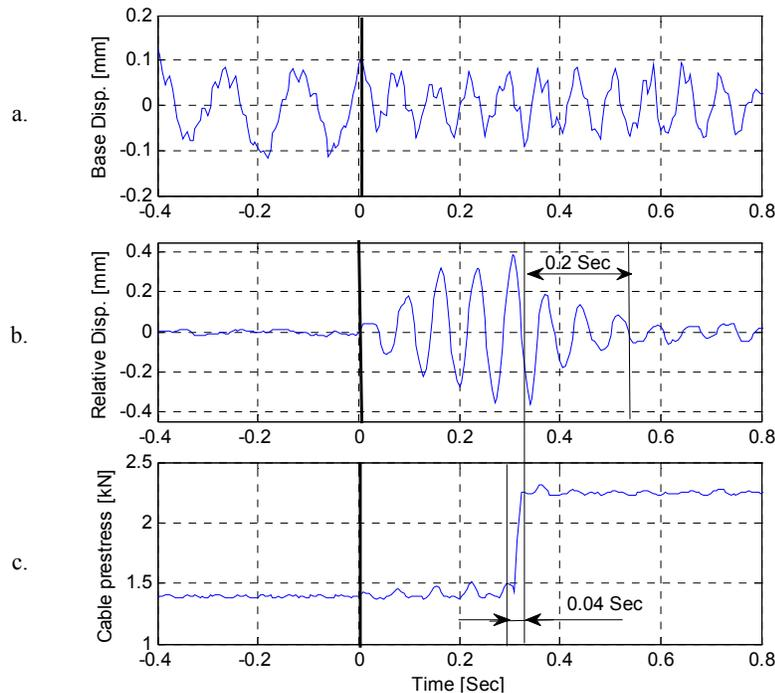
**Figure 5-33. a. Base displacement during test b. Base-Platform relative displacement c. Cable force in the VSM-C**
