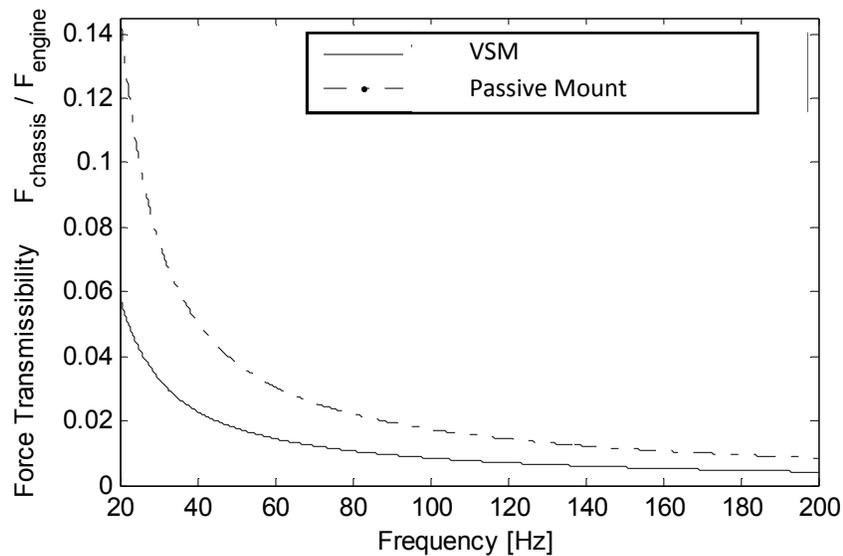
**Figure 3-11 Force transmissibility of VSM and the passive mount**
