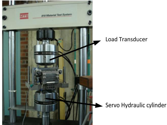
**Figure 5-14. Set-up on the Dynamic Testing machine**
