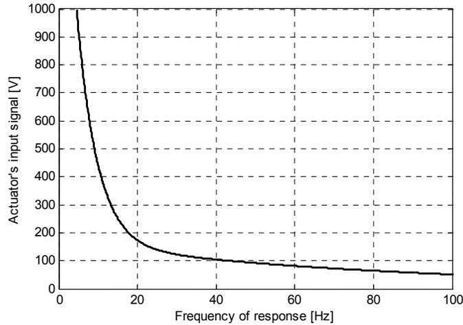
**Figure 5-11. Frequency response of the amplifier for the selected actuator**
