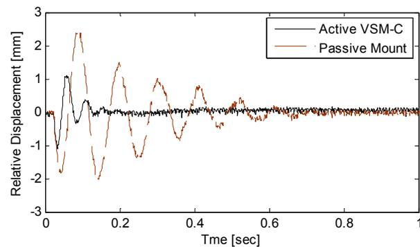
**Figure 5-32. Relative displacements of the passive mount and VSM-C caused by a shock**
