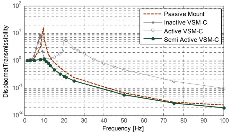
Figure 5-34. The control criterion of the semi-active VSM-C
