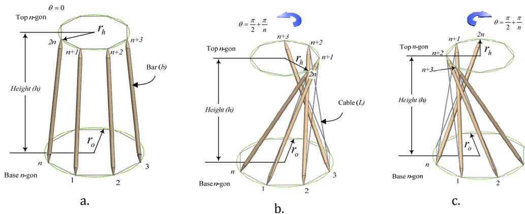
**Figure 4-4. How an  $n$ -gon tensegrity prism ( $n$ -gon TP) is built a.  $n$ -gon truncated pyramid b. Right-hand TP (studied in this chapter) c. Left-hand TP**
