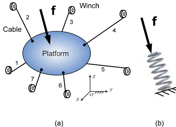
Figure 2-8. Cable-driven mechanism can work as a spring.
