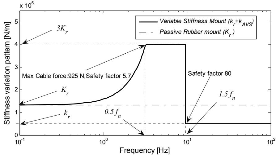
Figure 3-7 Frequency dependent stiffness of VSM
