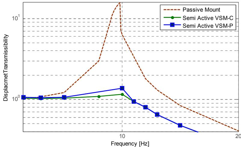
Figure 5-36. Transmissibility comparison between semi-active VSM-C and semi-active VSM-P
