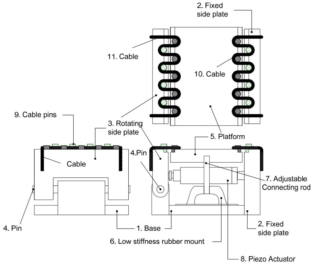
**Figure 5-1 Components of the designed and built antagonistic variable stiffness mount (VSM) that uses cable**
