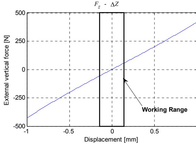
Figure 4-12. Force-Displacement relation of the square TP spring (Prestress 2200 N)
