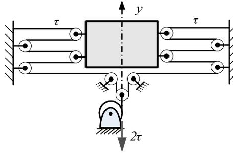
**Figure 3-3 The number of the cable forces can be increased to increase the maximum prestress stiffness or the range of the controllable stiffness**
