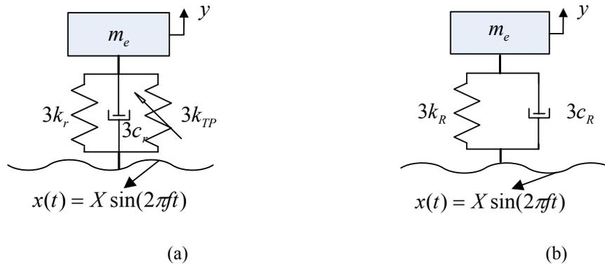
**Figure 4-9. a. A one DOF engine vibration model with VSM, b. A one DOF engine vibration model with PM**
