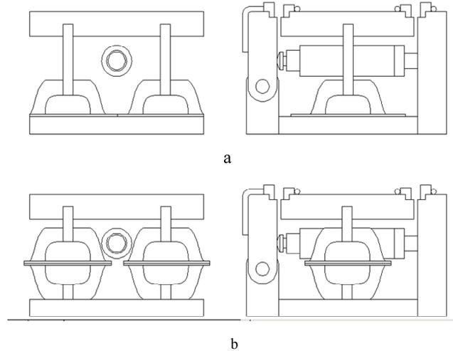
**Figure 5-13. Arrangement of the rubber mounts for a. representing the passive mount (without using the AVS) b. VSM**
