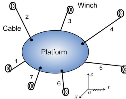
Figure 2-7. Cable-driven mechanism with one degree of kinematic redundancy
