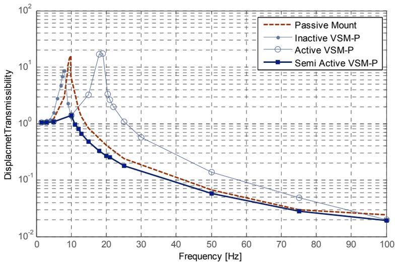
Figure 5-35. How the Semi-active VSM-P works and its comparison with an equivalent passive mount
