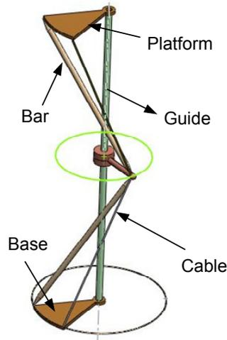
**Figure 2-5. An AVS made with a kinematically singular prestressed mechanism other than cable-driven mechanism and tensegrity**
