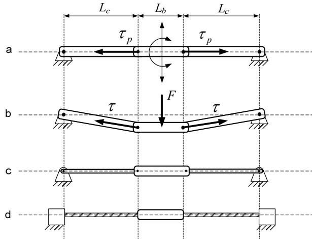
**Figure 2-4. a. Four-bar mechanism in a kinematically singular and prestressable configuration b. The same mechanism deflected under external load c. Side links are substituted with thinner links that have lower elasticity d. To eliminate joints, cables are used as side links**
