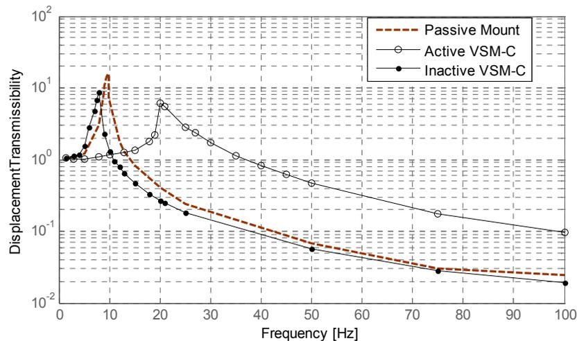
**Figure 5-27. Measured displacement transmissibility of the VSM-C in different configurations**
