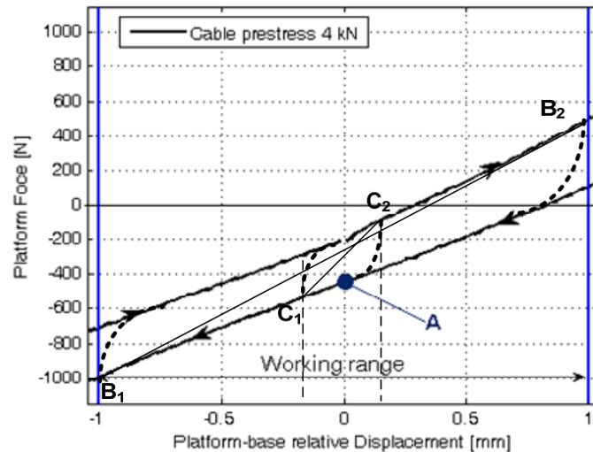
**Figure 5-19. How the hysteresis in a VSM-C affects on its dynamic stiffness**
