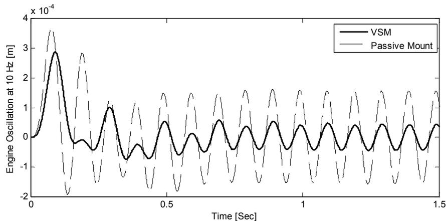
**Figure 3-9 The oscillation of the engine**
