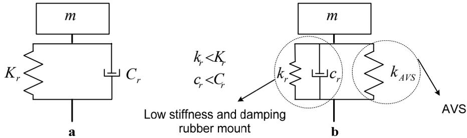
Figure 2-16. Schematics of one DOF vibrating system a. with passive mount b. with variable stiffness spring mount (VSM)
