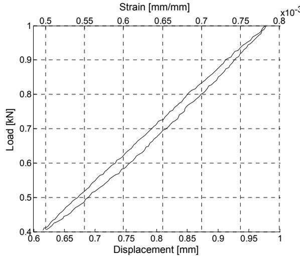
**Figure 5-7. Hysteretic effect caused by the internal friction of the wires**
