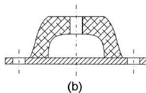
**Figure 4-8. a. Variable Stiffness engine Mount(VSM) made with a soft rubber mount and a square TP b. Regular passive engine mount (PM)**
