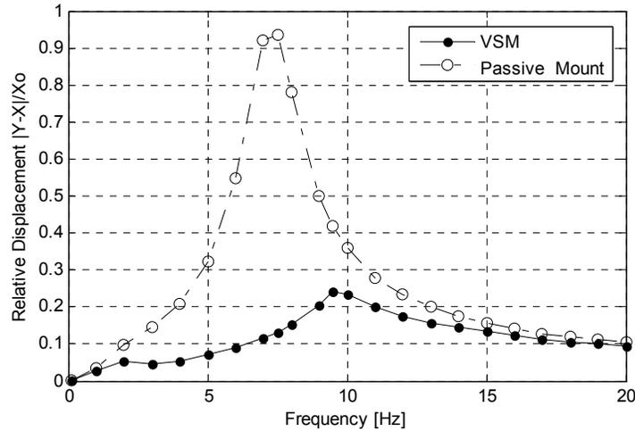
**Figure 3-10 Relative displacement of the engine and chassis**
