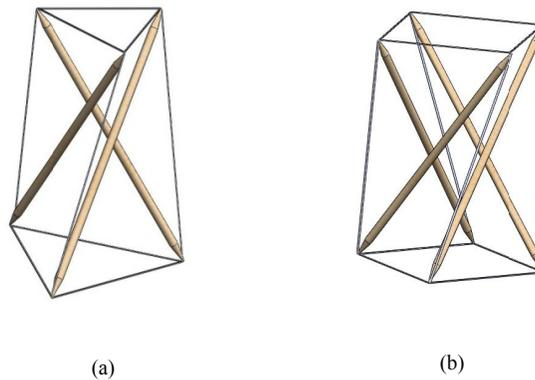
**Figure 4-3. Two tensegrity Prisms (TP) a.Triangular TP b. Square TP**
