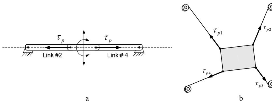
**Figure 2-2 Antagonistic stiffness of a 4-bar linkage**
