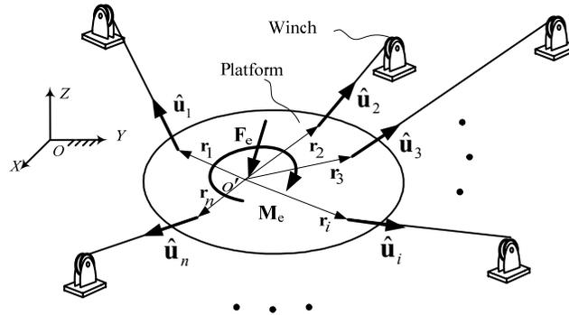
**Figure 3-1 General model of a cable-driven mechanism**
