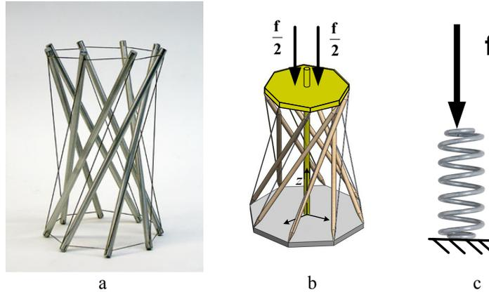
**Figure 2-12. a. An Octagonal Tensegrity Prism (Courtesy K.Snelson) b. Spring developed by tensegrity prism, this spring can works as a translational spring c. Translational coil Spring**
