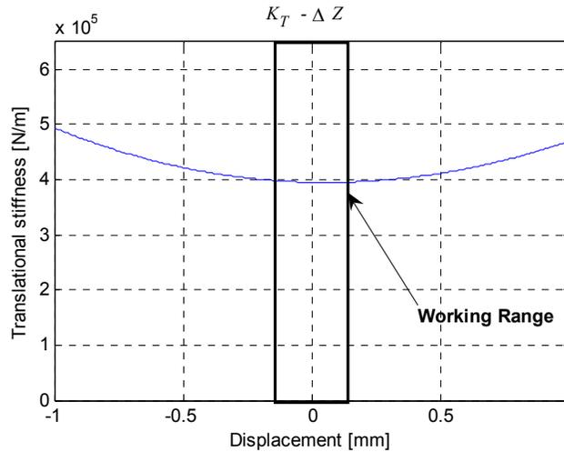
Figure 4-13. Stiffness change with displacement of the square TP spring (Prestress 2200 N)
