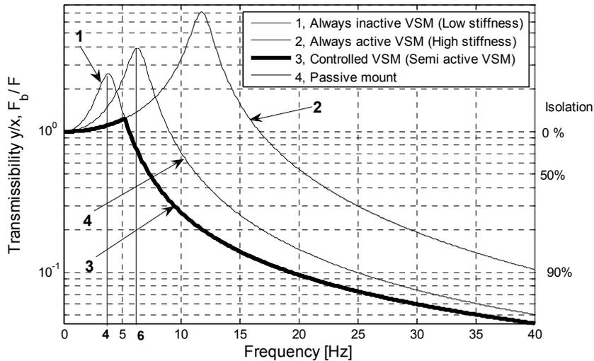
Figure 2-17. Semi-active vibration-control by varying the stiffness
