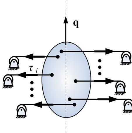
**Figure 2-9. Desired configuration of a translational AVS.**
