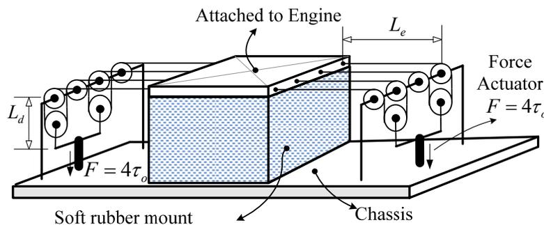
**Figure 3-5 Schematic of the VSM developed with cable-driven mechanism**
