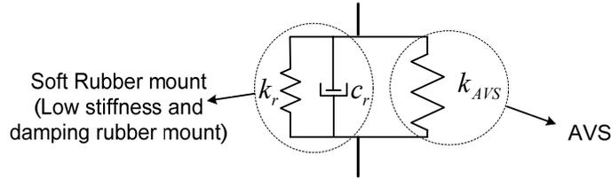
Figure 5-25. Model of the VSM-P used for predicting the transmissibility of the VSM-P
