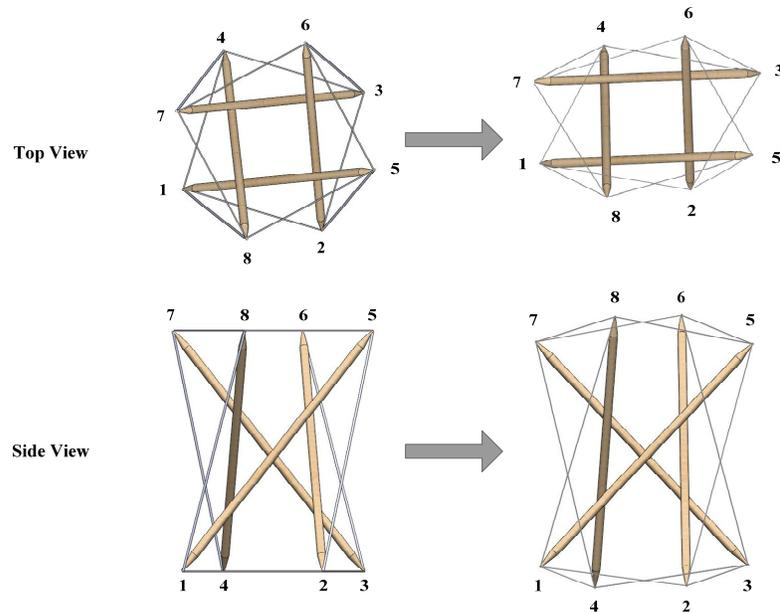
**Figure 4-5, Top and side views of the second FOIM of a square TP**
