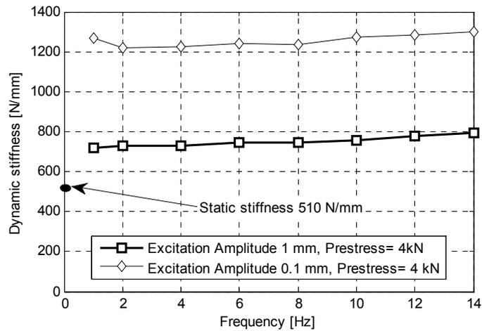
**Figure 5-18. Dynamic Stiffness of the active VSM-C, Prestress equals 4 kN, tested in different excitation frequencies**
