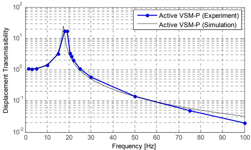
**Figure 5-30. Comparison between measured and simulated displacement transmissibility of VSM-P at high prestress level**
