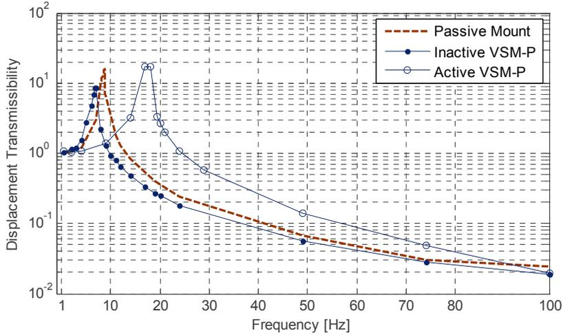
**Figure 5-29. Measured displacement transmissibility of VSM-P in different configurations**
