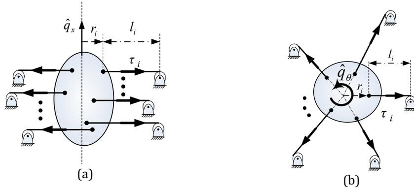
**Figure 3-2 Two possible mechanisms with zero elastic stiffness and maximum prestress stiffness along the shown directions**
