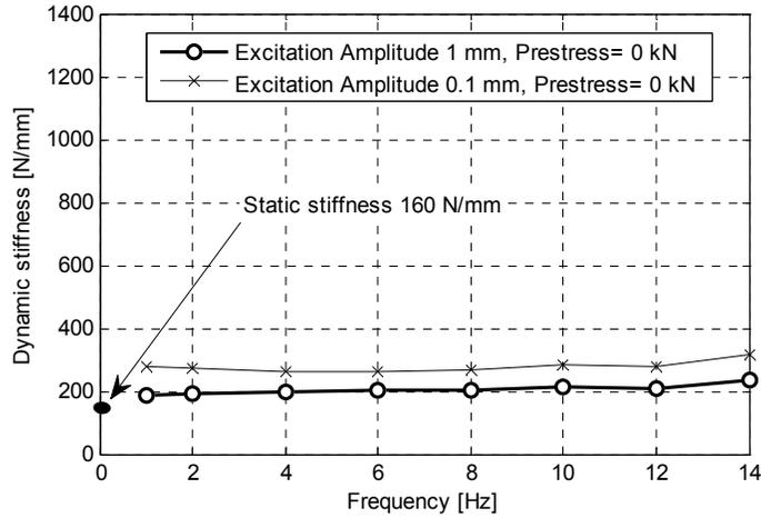
**Figure 5-17. Dynamic Stiffness of the inactive VSM-C Prestress equals zero, tested in different excitation frequencies**
