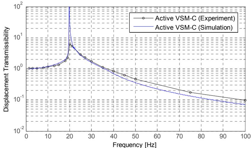
**Figure 5-28. Comparison between measured and simulated displacement transmissibility of the VSM-C at high prestress**
