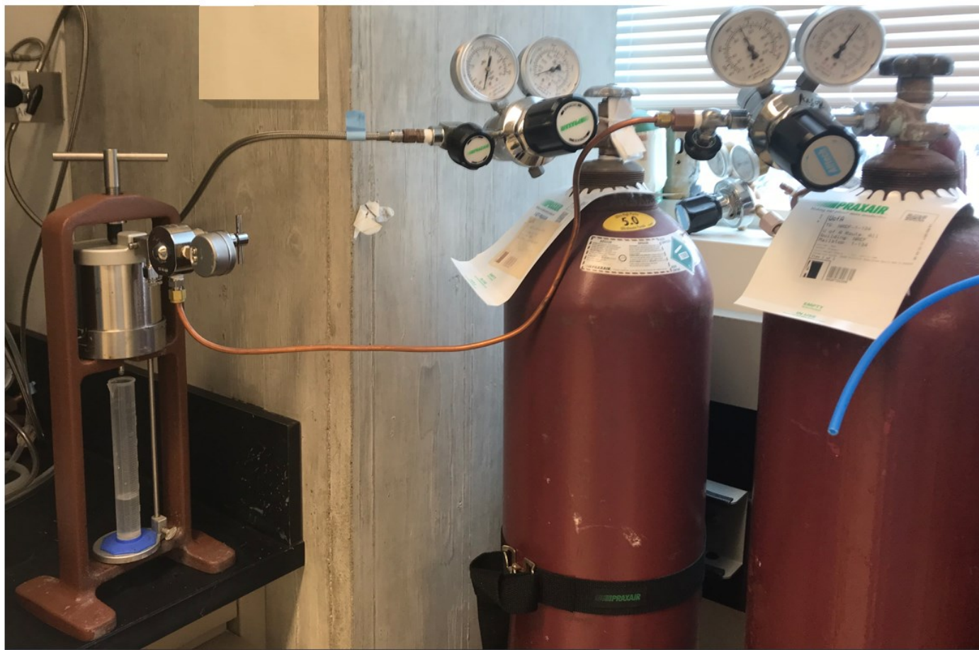
Figure B1. Pressure filter (OFITE; Bench-Mount Filter Press with Hose and Regulator; #140-31) used at Chapter 3 to increase the solids content of raw FFT to 50% (wt./wt.) at 100 psi.
