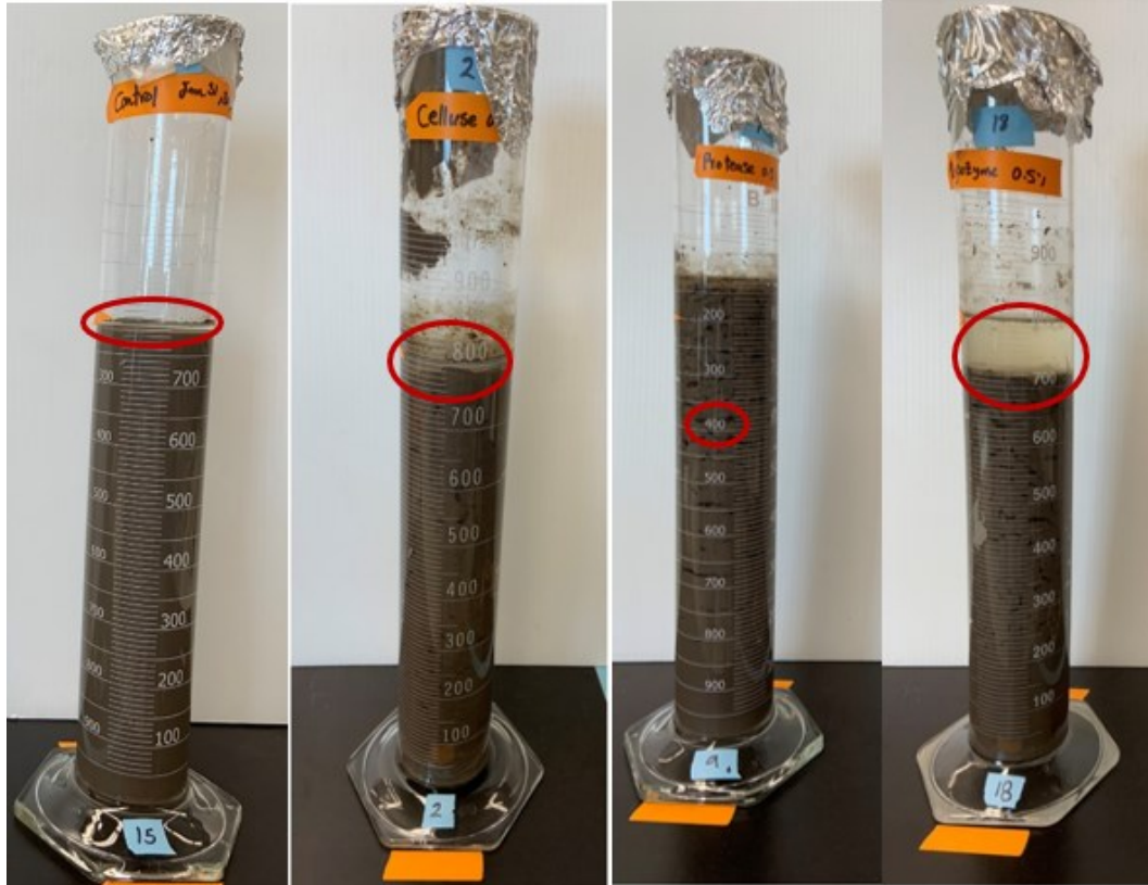
Figure 4.2. Different cracks appeared in the FFT columns treated with cellulase, protease, and lysozyme throughout the experiment compared to the control.
