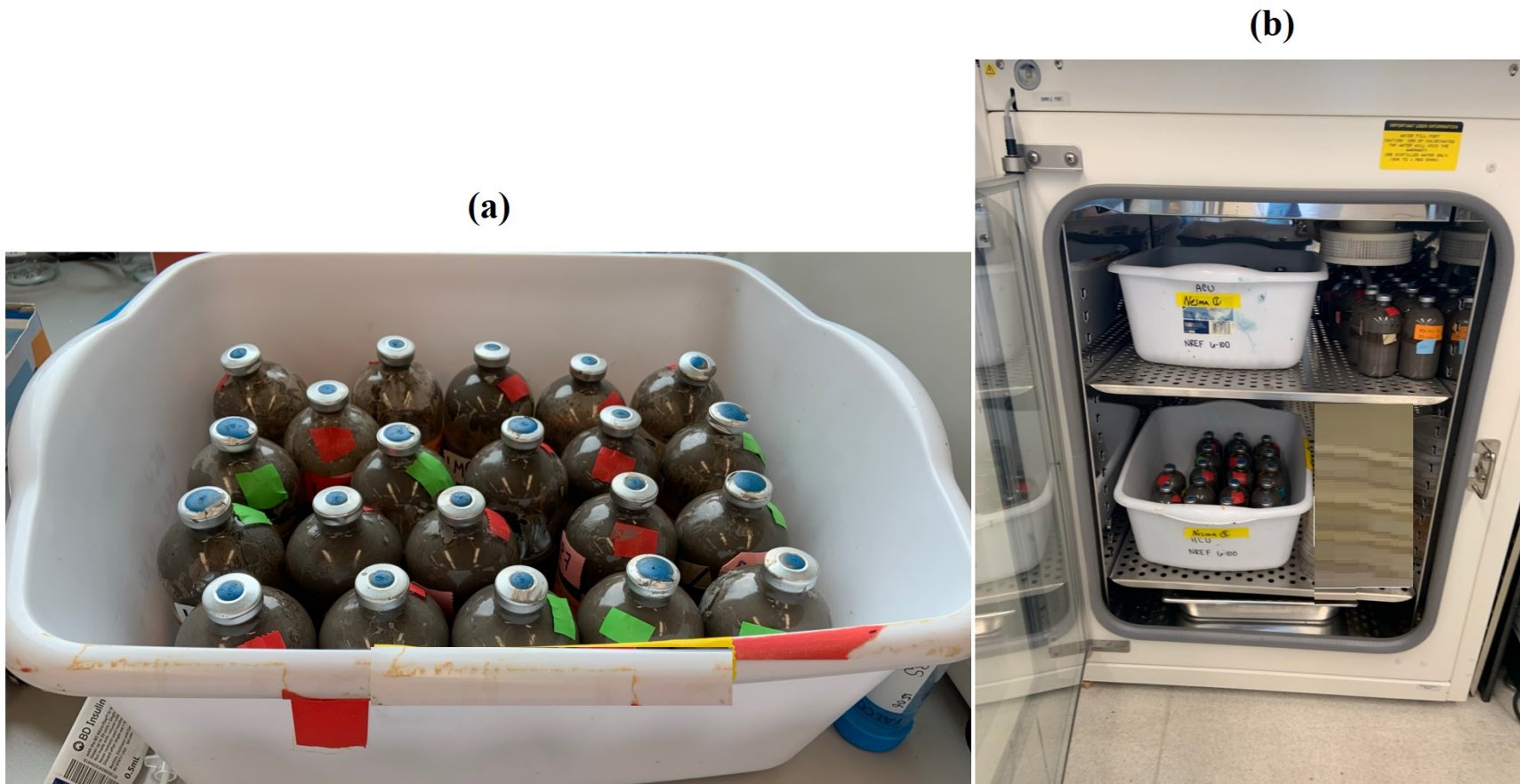
Figure B4. The experimental set-up for Chapter 5, (a) 158 mL microcosms consists of 65 mL FFT and 35 mL of anaerobic media control, treated with enzyme, lime or BES, (b) All the microcosms incubated at 30 °C incubator in dark conditions.
