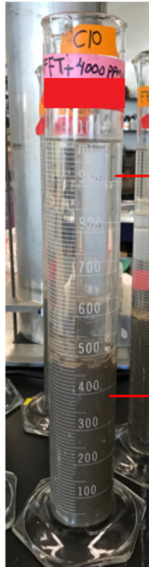
Figure B2. The experimental set-up for Chapter 3 consists of 500 ml lime treated or untreated FFT (50% solids) covered with 500 ml Raw synthetic OSPW. All columns were open to the atmosphere.
