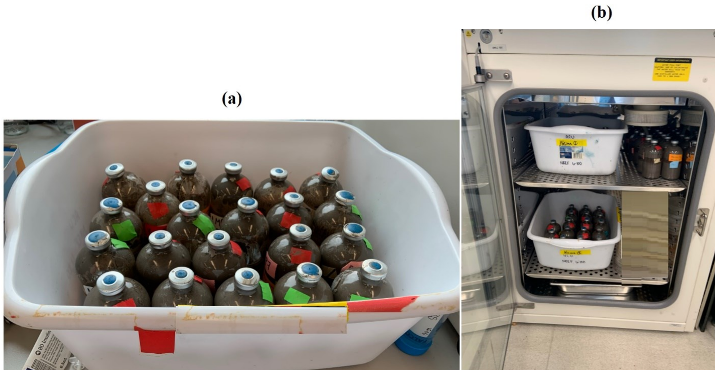
Figure 5.1. Photographs of experimental setup (a) 158 mL microcosm consists of 65 mL FFT and 35 mL of anaerobic media control, treated with enzyme, lime or BES, (b) the microcosms incubated in dark conditions at 30 °C.
