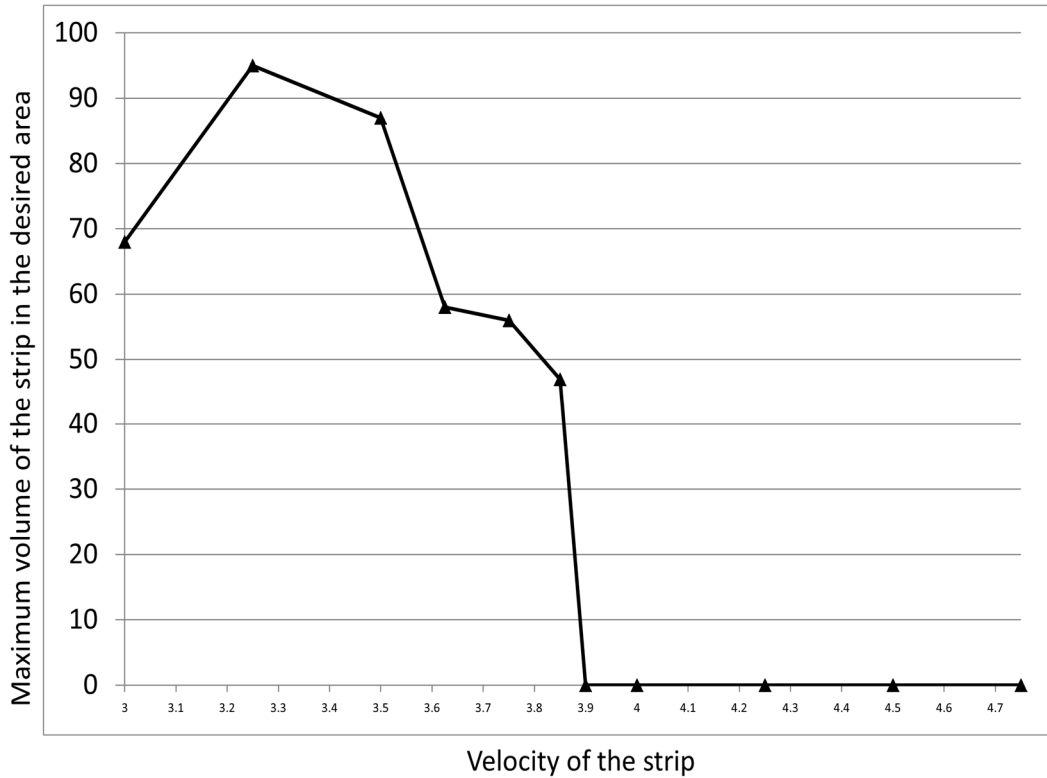
Figure 6-12. Maximum percent volume of the strip whose temperature is in the desired zone for each velocity
