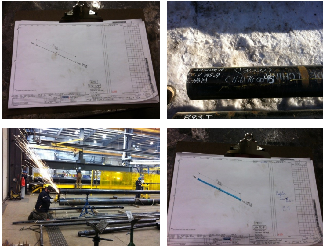
Figure 5-14 Fabrication process for pipe spool No.3
