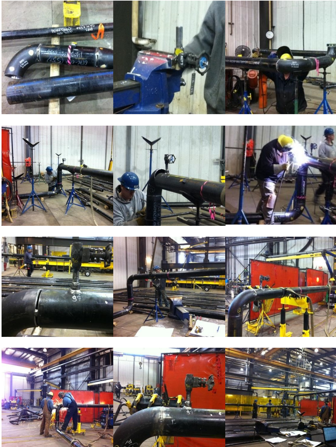
Figure 5-25 fabrication process for pipe spool No. 7
