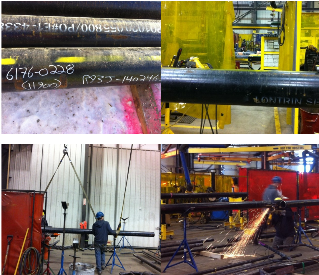
Figure 5-16 Fabrication process for pipe spool No. 4
