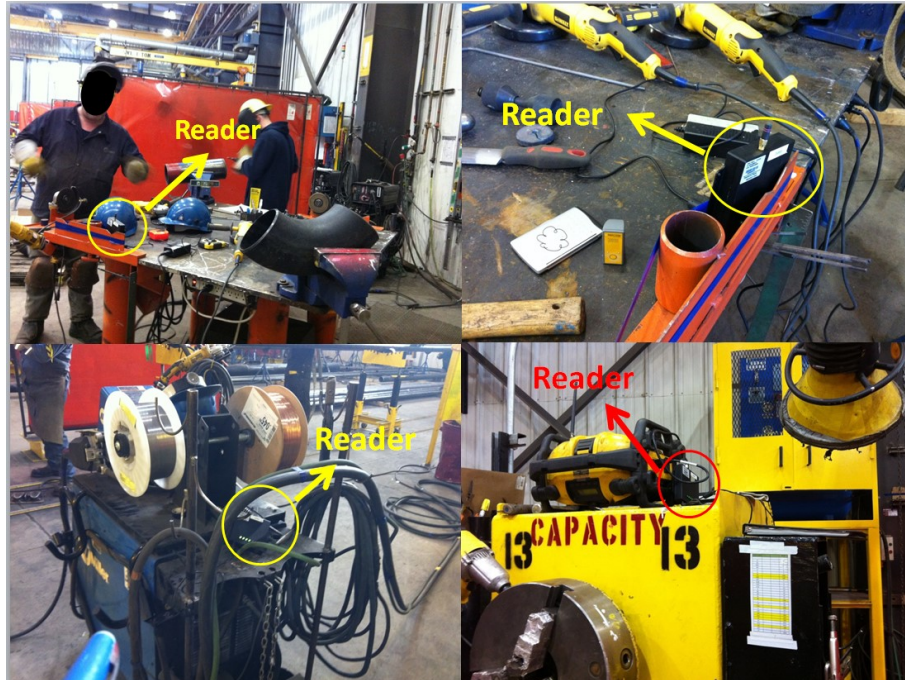
Figure 4-4 beacons placed at one fitting and three welding stations
