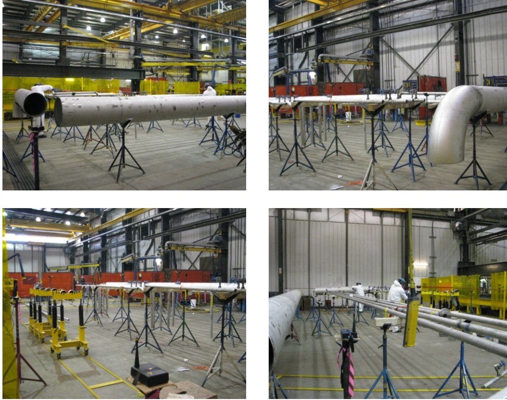
Figure 2-20 Different configuration of pipe spool fabrication in the test area
