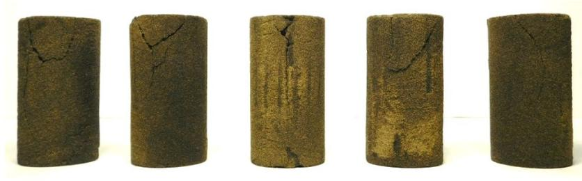
10%-Binder Saturation- 45° Layer Orientation- 250 μm Layer Thickness
