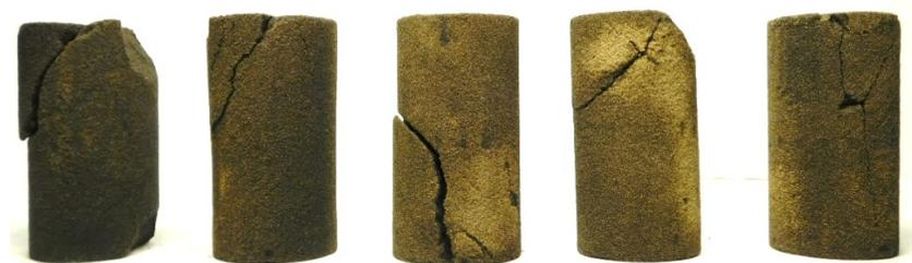
10%-Binder Saturation- 65° Layer Orientation- 250 μm Layer Thickness
