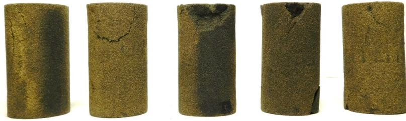
10%-Binder Saturation- 90° Layer Orientation- 250 μm Layer Thickness
