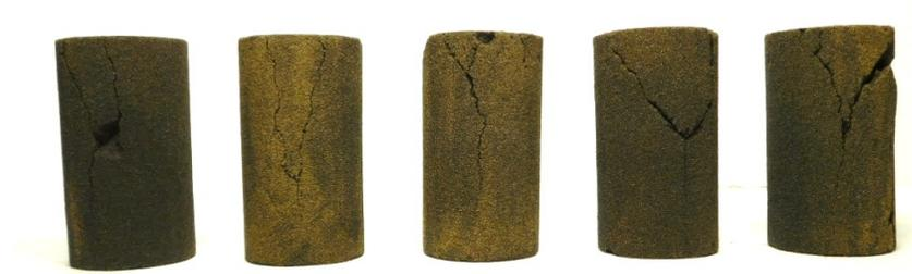
20%-Binder Saturation- 0° Layer Orientation- 250 μm Layer Thickness
