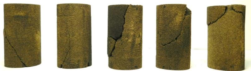
10%-Binder Saturation- 0° Layer Orientation- 400 μm Layer Thickness
