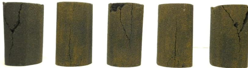
10%-Binder Saturation- 25° Layer Orientation- 250 μm Layer Thickness
