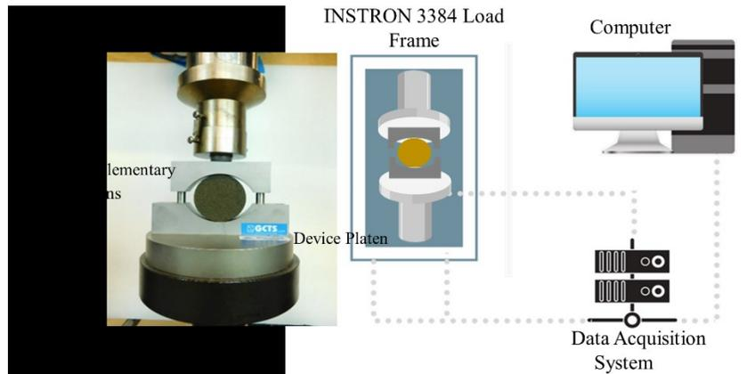
**Figure 3.6. Experimental Setup and Data Logging configuration for Brazilian Tests on 3DP Specimens**
