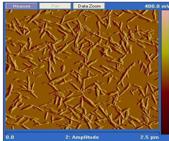
Figure 4.1. An AFM image of CNC particles
