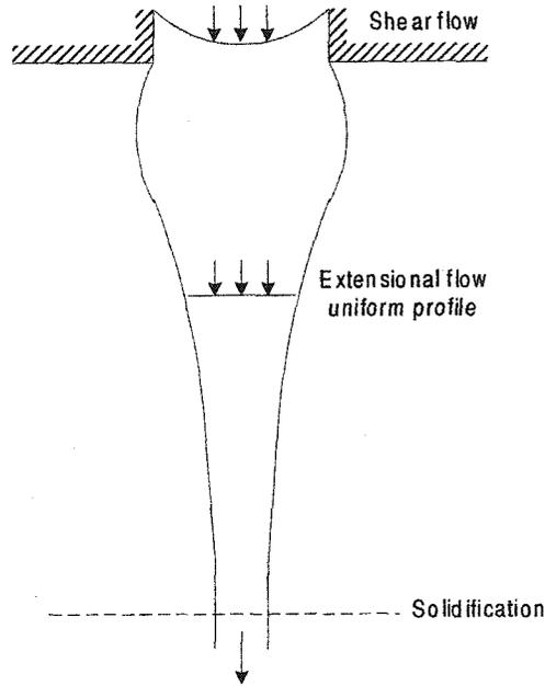
Figure 1.3: Melt spinning
