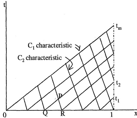
Figure 5.4: State variable prediction along characteristics
